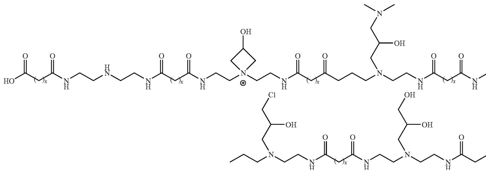
Structure 2 shows a polymer with one end-group based on a di-acid group and the other end-group based on a nitrogen group:
