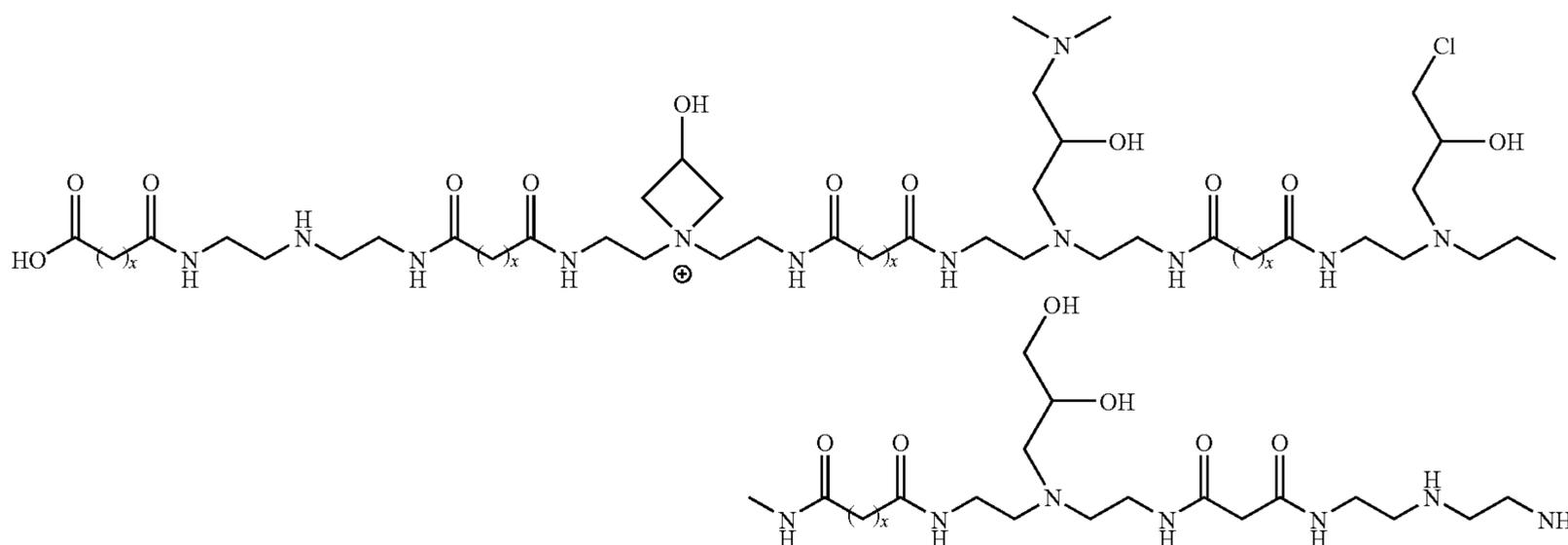
Note that although both structures are based on DETA, other polyamines may be used to form this polymer, including those, which may have tertiary amide side chains.
