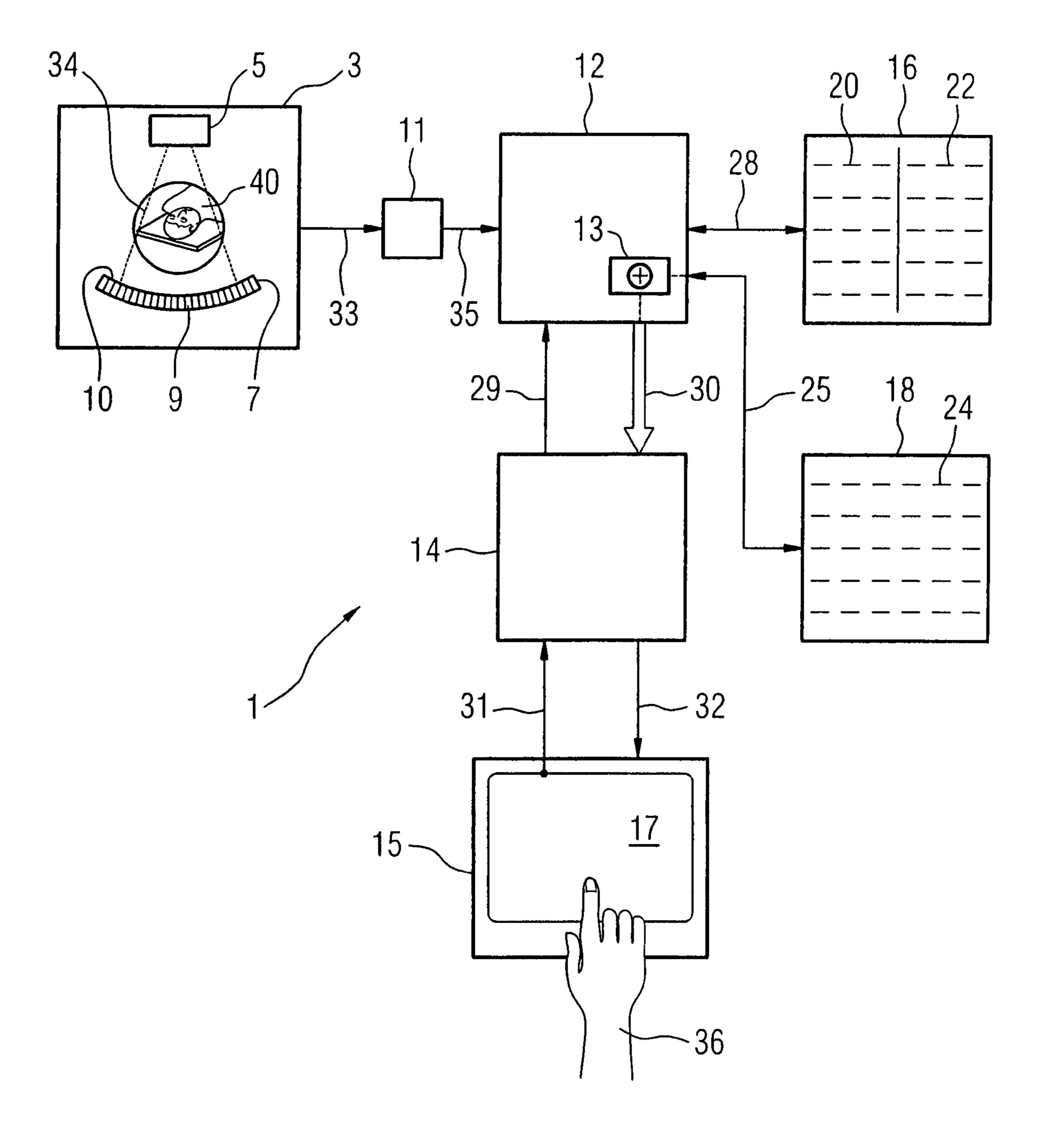
DETECTING APPARATUS AND METHOD FOR DETECTING AN OBJECT BY MEANS OF A PROJECTION THROUGH THE OBJECT BY MEANS OF X-RAYS, AND A CONTRAST—AND NOISE-OPTIMIZED QUANTUM COUNTING DETECTOR
