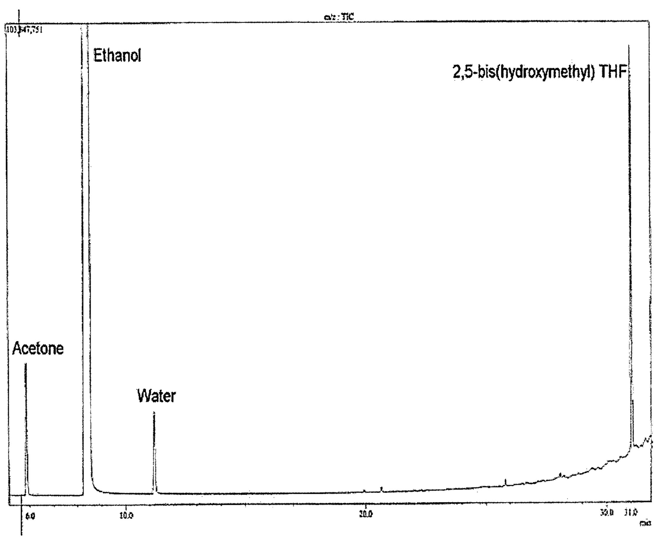
GC spectrum of product produced from hydrogenation of 5-hydroxymethyl furfural T=200°C, P=1500psig H<sub>2</sub>, Catalysts =10% run in ethanol.
