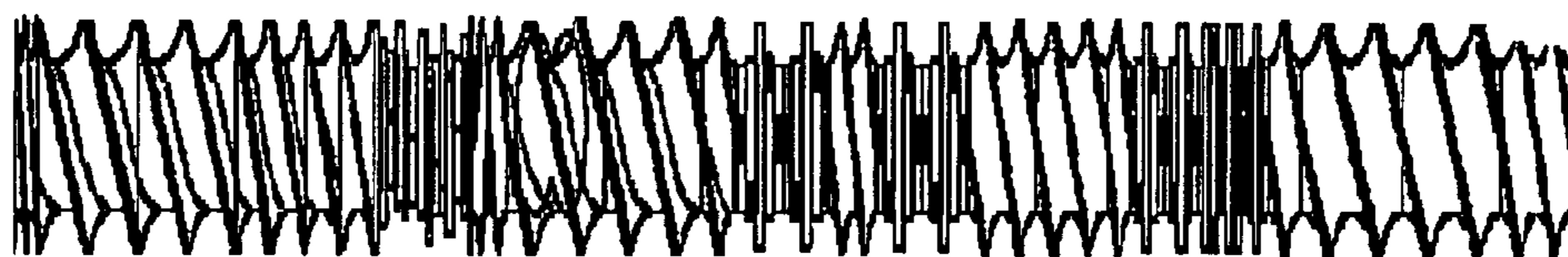
Screw configuration II with three kneading zones
