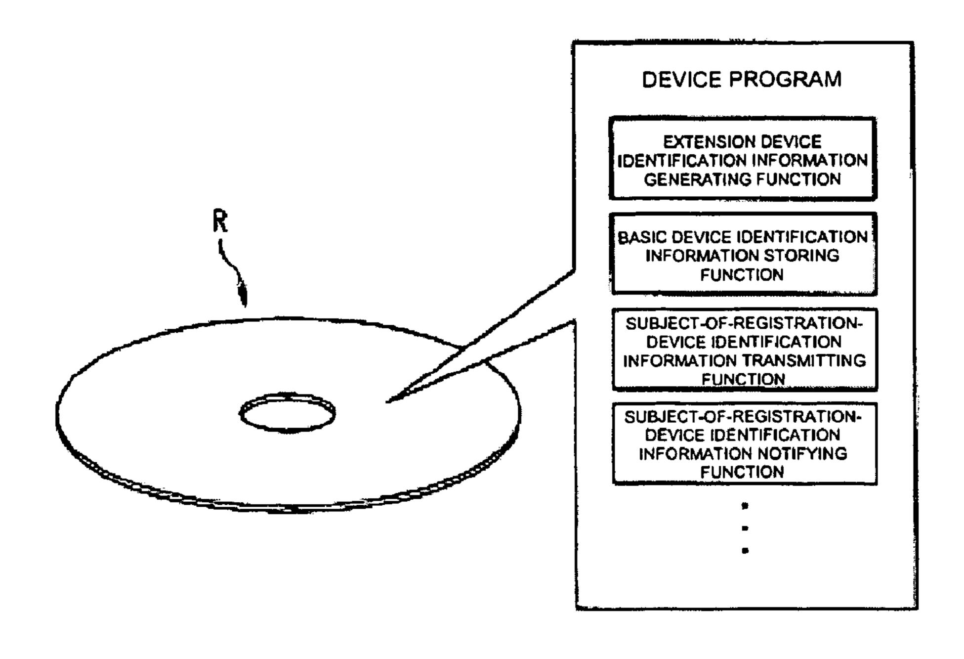
DEVICE IDENTIFICATION INFORMATION MANAGING SYSTEM AND METHOD FOR COMMUNICABLY CONNECTING BETWEEN A NETWORK DEVICE AND A DEVICE MANAGING TERMINAL UNIT THAT MANAGES THE NETWORK DEVICE
