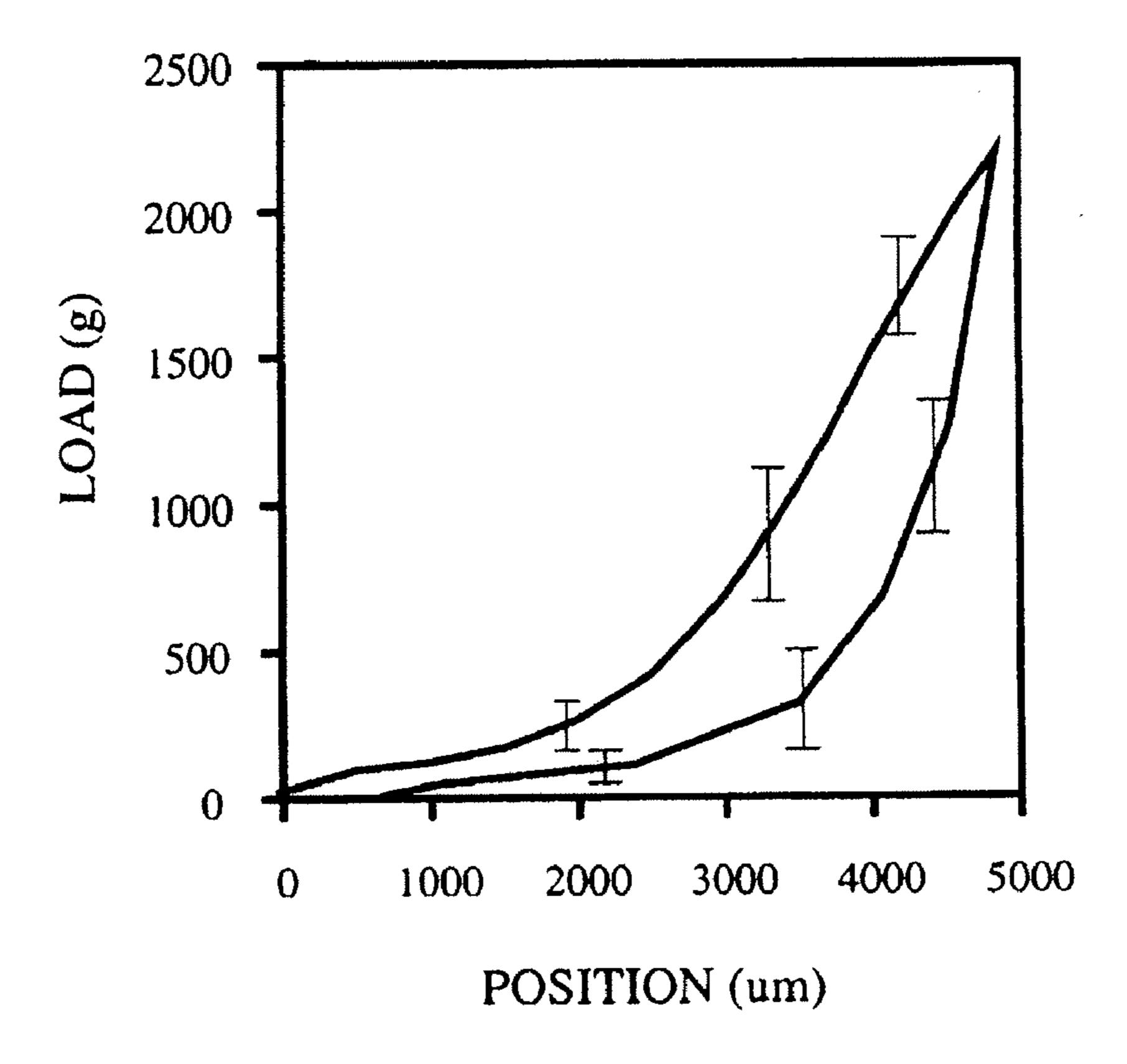
Ramp Tension with Release Speed: 200 um/s
