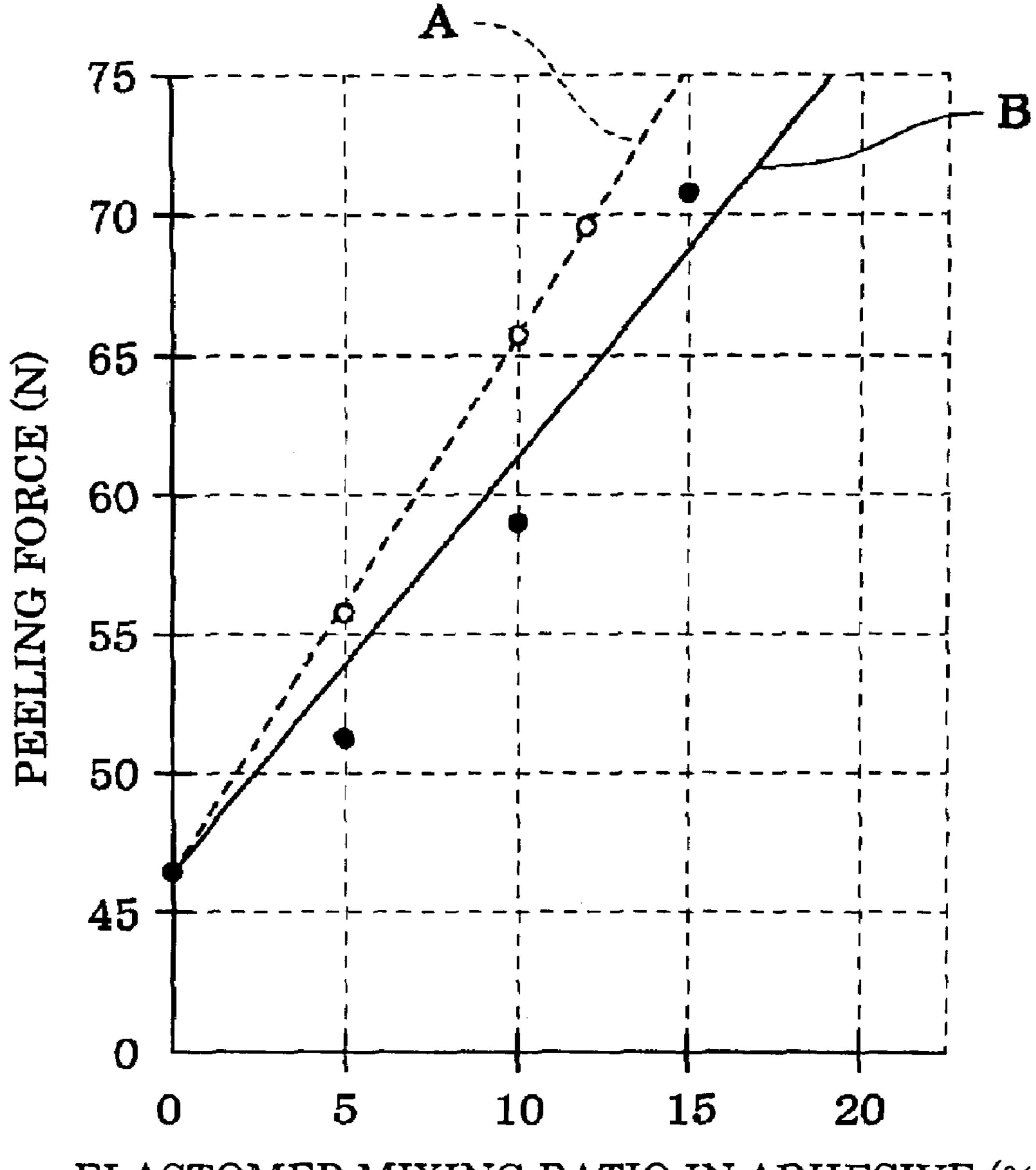
ELASTOMER MIXING RATIO IN ADHESIVE (%)
