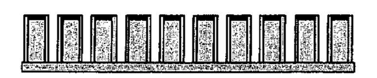
Metal Coated polymer columns after electroless plating
