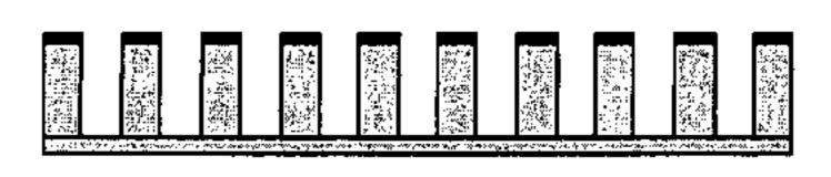
Pl columns on Silicon after dry etching and cleaning
