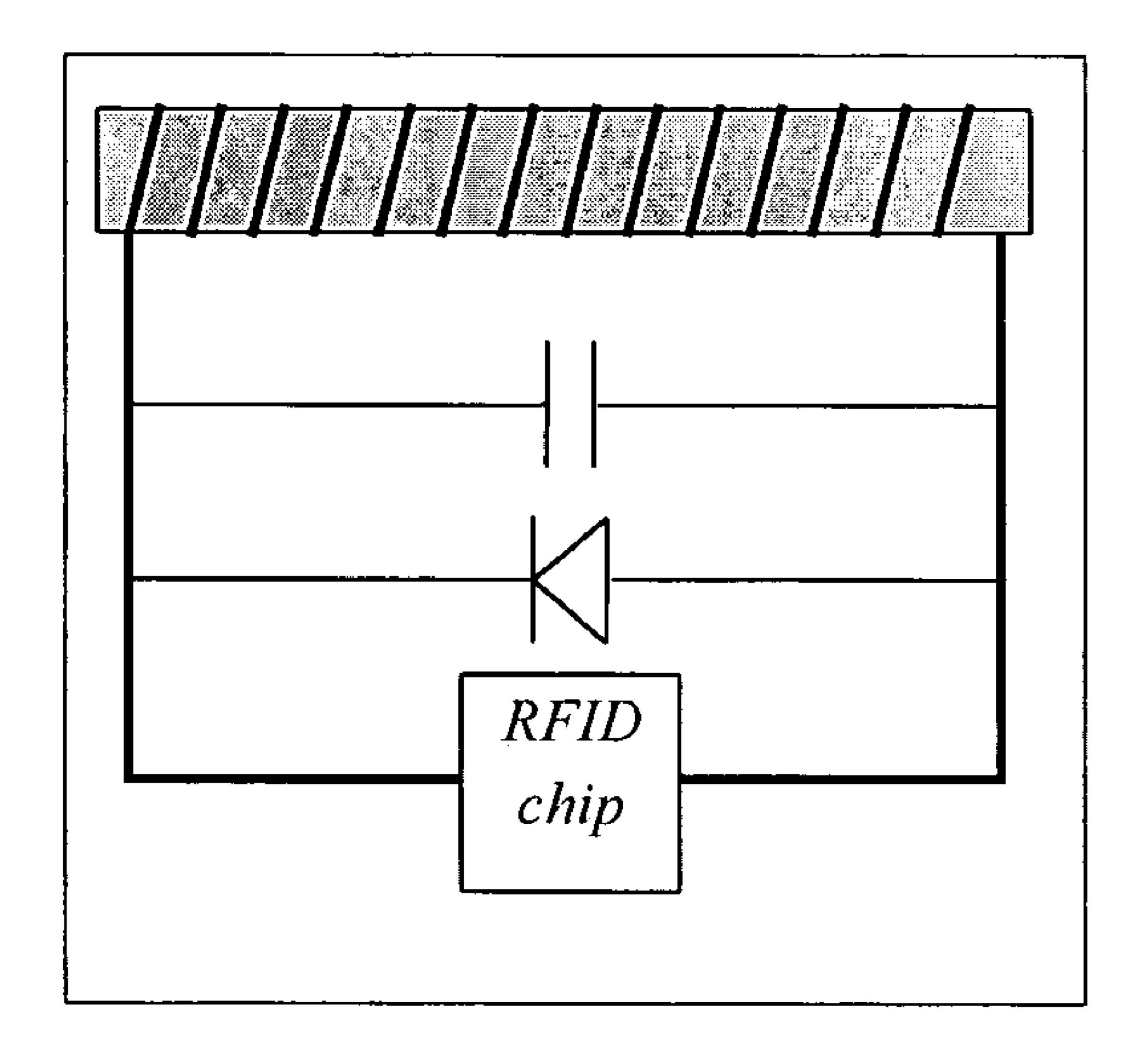
MEANS FOR MEASURING CHANGE IN RESONANT FREQUENCY
