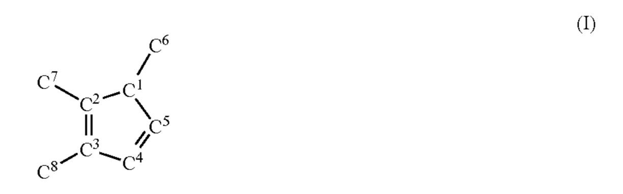
wherein C<sup>1</sup> to C<sup>8</sup> are carbon atoms constituting a fullerene skeleton in which C<sup>6</sup> to C<sup>8</sup> are independently bonded to an organic group having 1 to 50 carbon atoms, and C<sup>1</sup> is bonded to a substituted or unsubstituted alkyl group having 1 to 20 carbon atoms.
