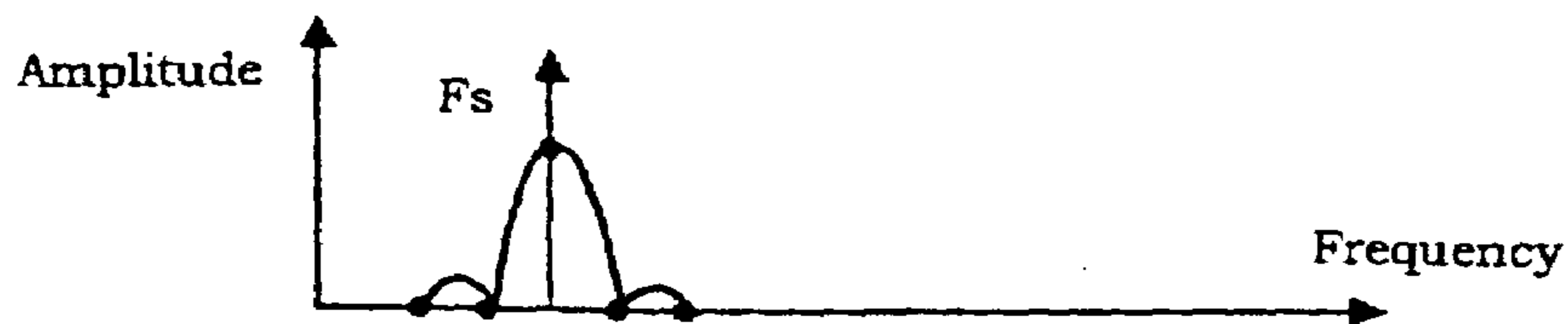
Figure 10(f) Data Spectrum Modulated onto Sub-Carrier
