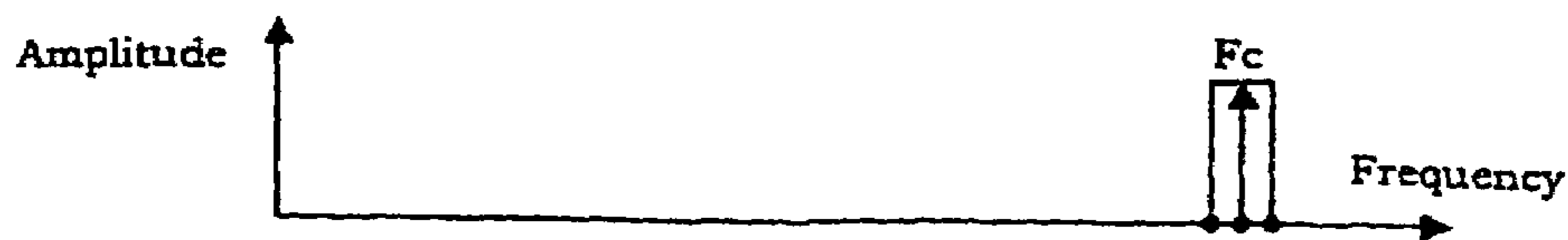
Figure 19(b): Carrier Modulated with Data
