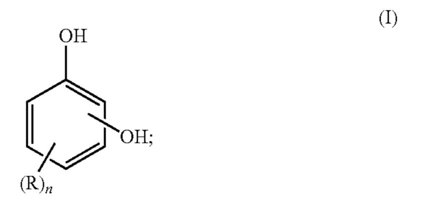
wherein R is a hydrogen atom or an aliphatic functionality having 1 to 6 carbon atoms and n is an integer having a value of 1 to 4.
