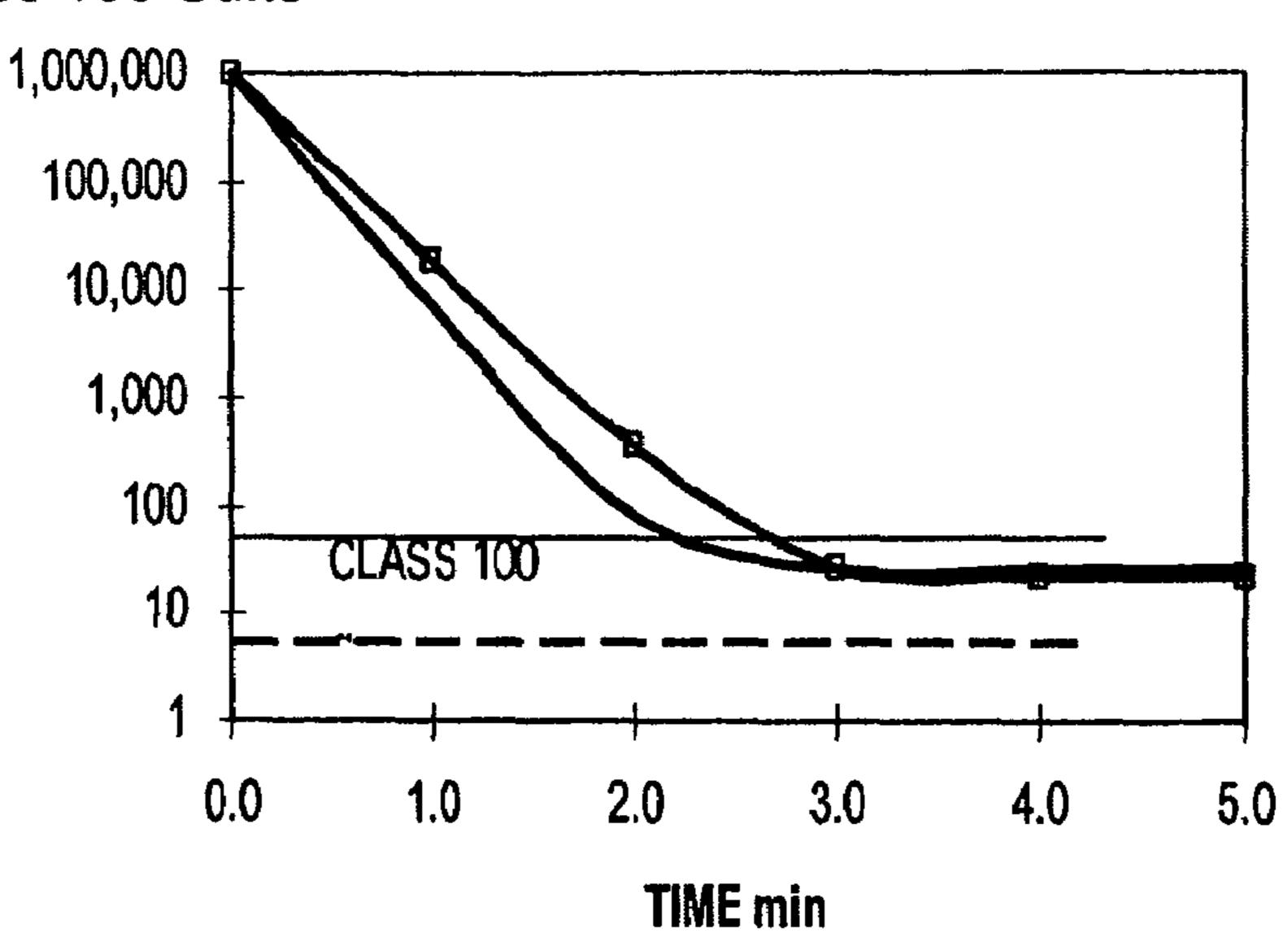
This graph shows the computer analysis (projected room performance.) the chart shows how fast a room cleans up after being initially contaminated. This is an important design parameter since there is always periodic step regression of contamination into the room.
