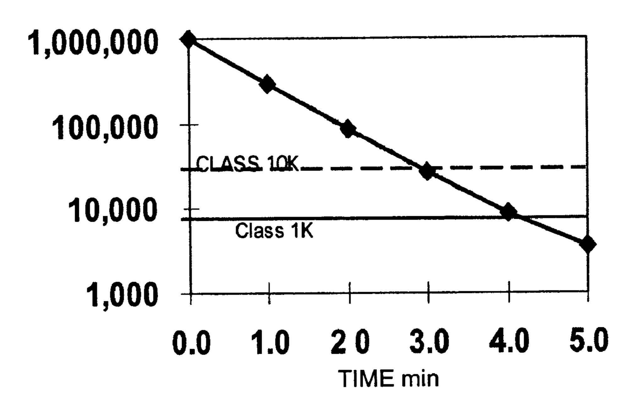
This graph shows the computer analysis (projected room performance.) the chart shows how fast a room cleans up after being initially contaminated. This is an important design parameter since there is always periodic step regression of contamination into the room.
