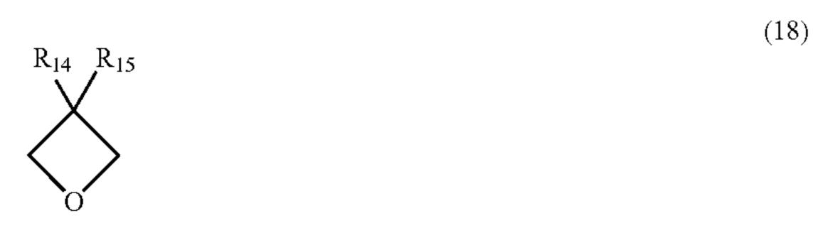
In this formula, R<sup>14</sup> and R<sup>15</sup> are the same or different and each represent a divalent organic group having 1 to 20 carbon atoms and at least one constituent atom selected from the group consisting of hydrogen, oxygen, and nitrogen.
