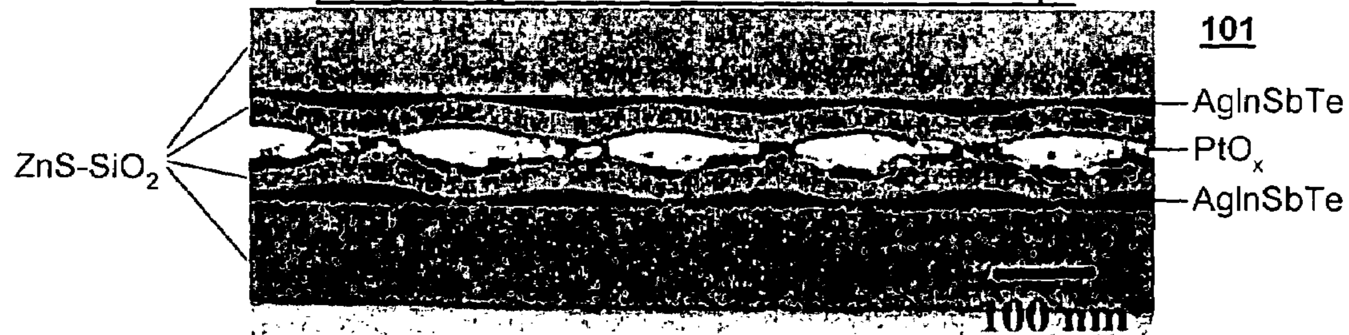
Picture of conventional super resolution optical disc taken using transmission electron microscope
