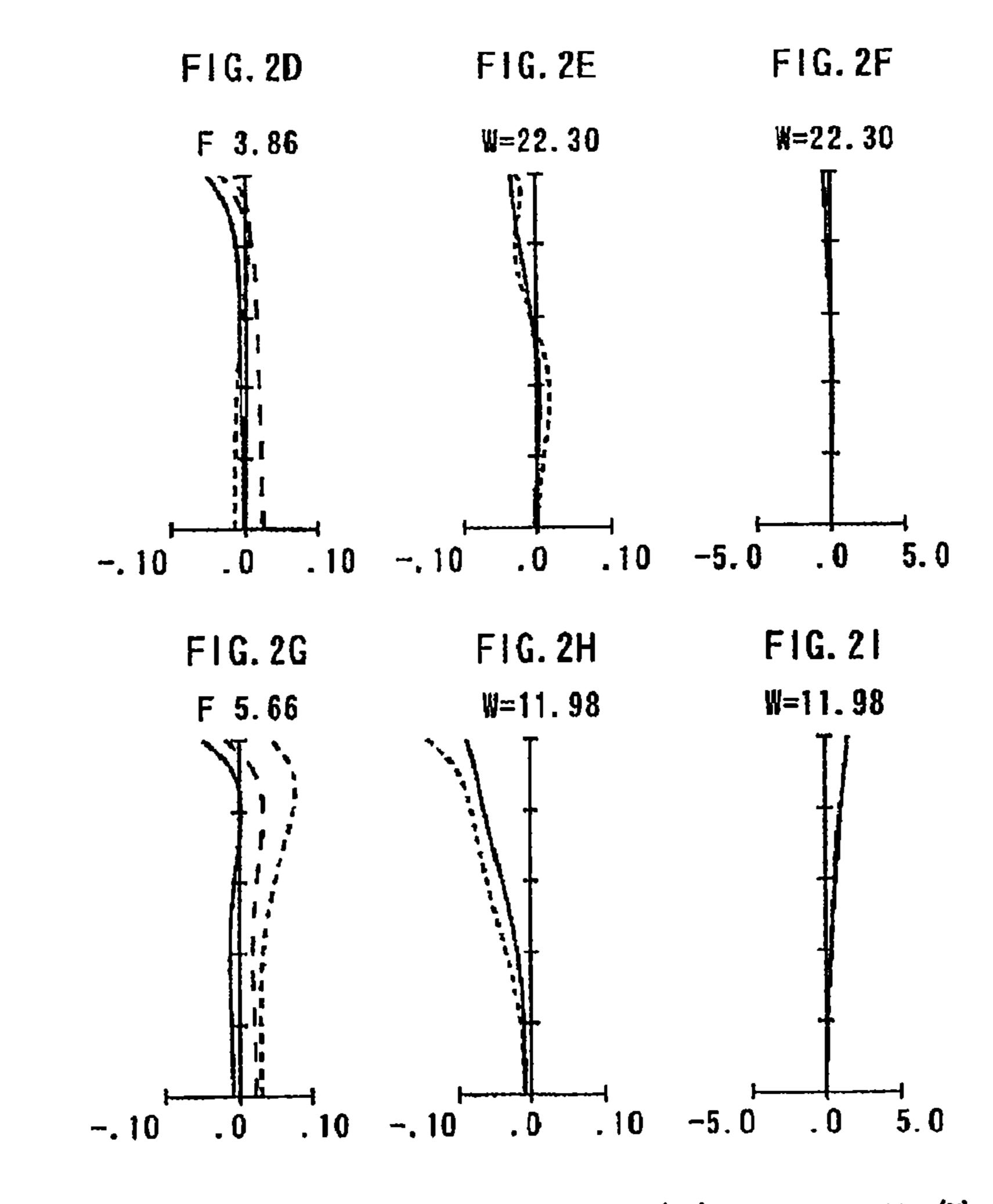
SPHERICAL ABERRATION (mm) ASTIGMATISM (mm) DISTORTION (%)
