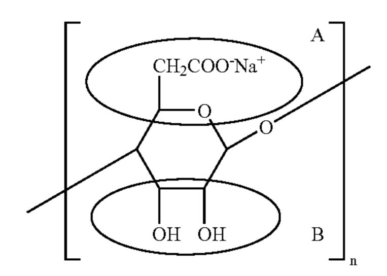
With respect to Formula 1, a structure of the carboxymethyl cellulose-based binder is shown where A is a hydrophilic binding site capable of binding with water, and B is a lipophilic binding site capable of binding with a carbonaceous material. The presence of the hydrophilic binding site that is substituted with a carboxymethyl group may increase the water solubility of the binder.
