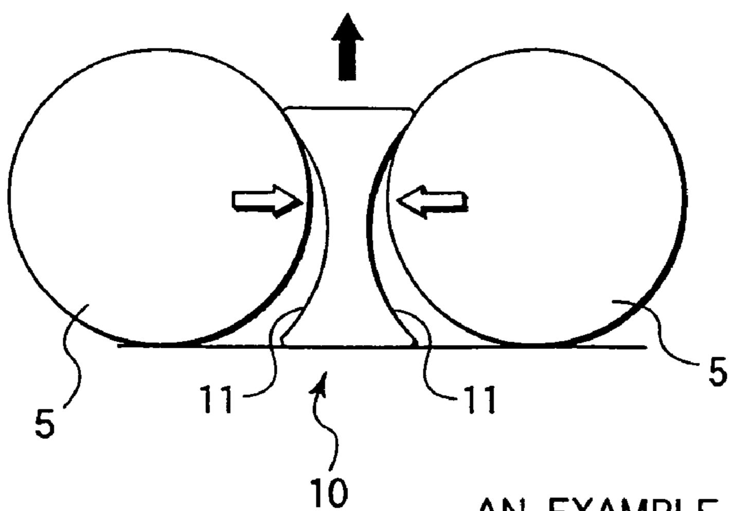
AN EXAMPLE IN WHICH RETAINING PIECE OUTSIDE DIAMETER IS EQUAL TO OR MORE THAN 0.5 TIMES DW
