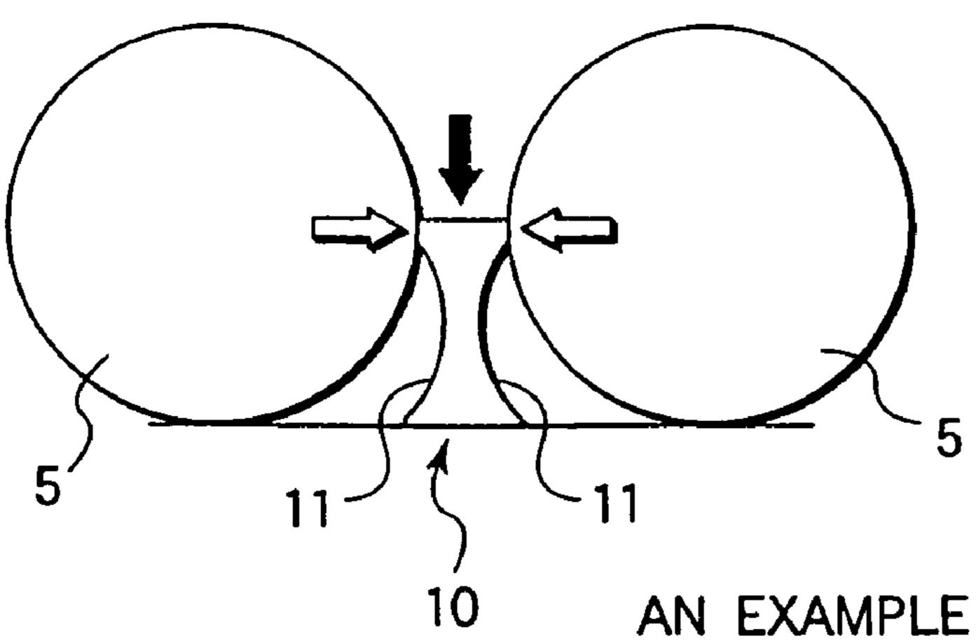
AN EXAMPLE IN WHICH RETAINING PIECE OUTSIDE DIAMETER IS EQUAL TO OR MORE THAN 0.5 TIMES DW
