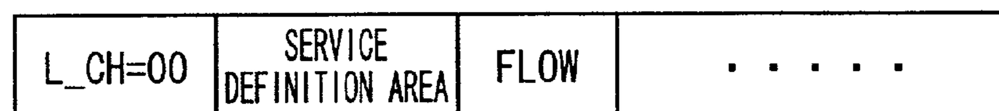
FIG. 10B ACL PAYLOAD HEADER EXAMPLE 2
