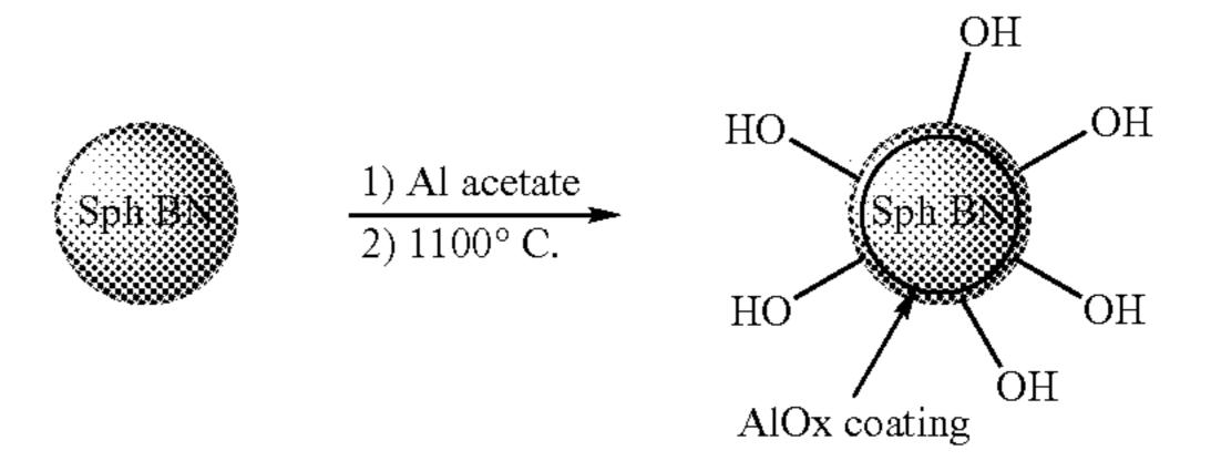
Surface Functionalizing BN with a Coupling Agent: The BN powder (either uncoated or optionally coated with a 1<sup>st</sup>
