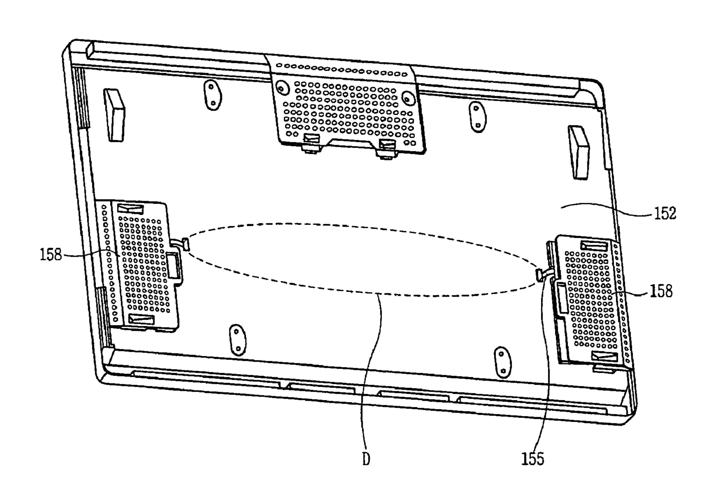
LCD MODULE HAVING INVERTER POWER SUPPLY WITH MASTER/SLAVE PORTIONS INTERCONNECTED BY FLEXIBLE FLAT CABLE MOUNTED ON INNER SURFACE OF LOWER COVER AND WHERE MASTER/SLAVE PORTIONS AND CORRESPONDING SIDES OF POWER SUPPLY LINE ARE EXPOSED ON OUTER SURFACE OF LOWER COVER
