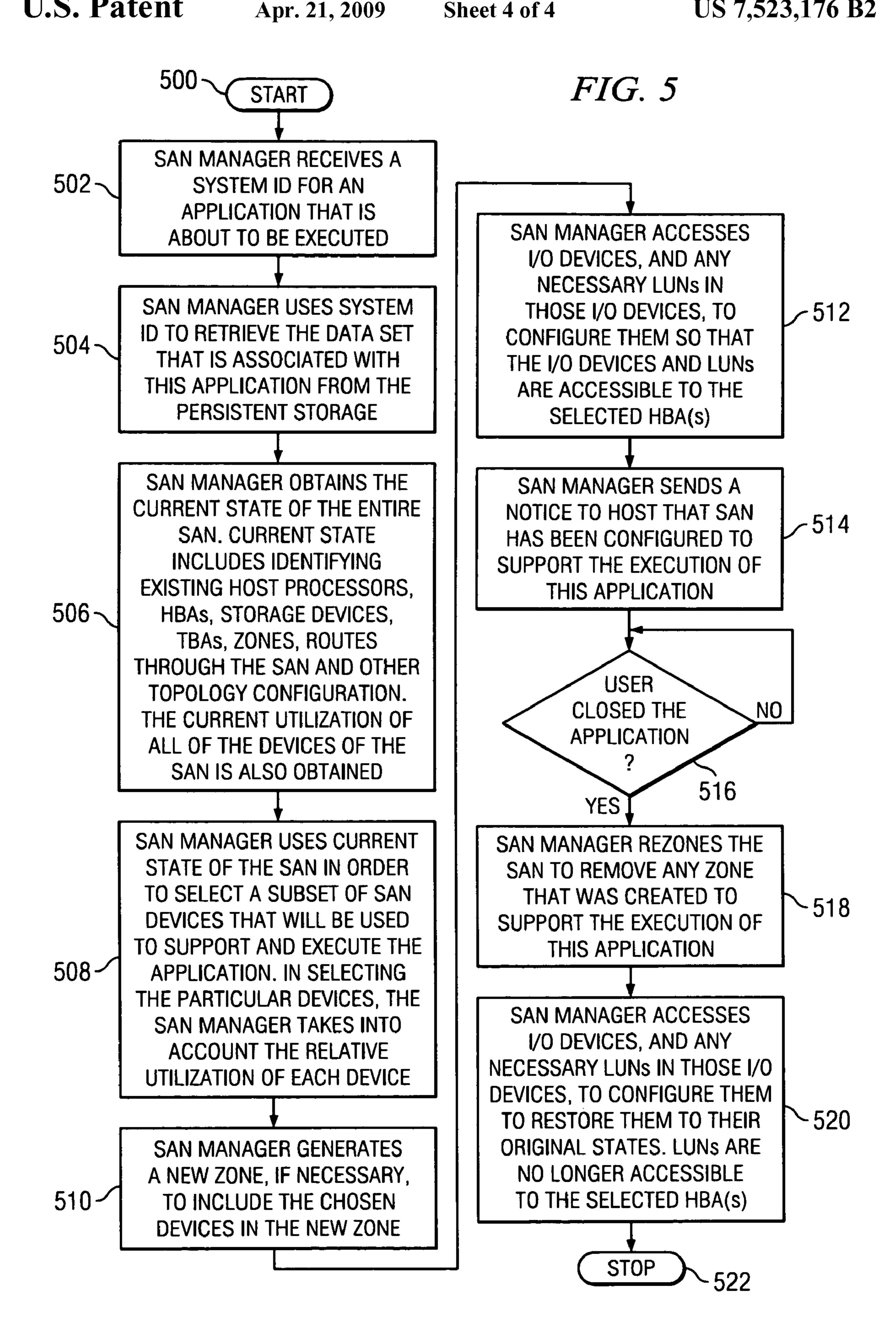
METHOD, APPARATUS, AND COMPUTER PROGRAM PRODUCT FOR RECONFIGURING A STORAGE AREA NETWORK TO SUPPORT THE EXECUTION OF AN APPLICATION AUTOMATICALLY UPON EXECUTION OF THE APPLICATION
