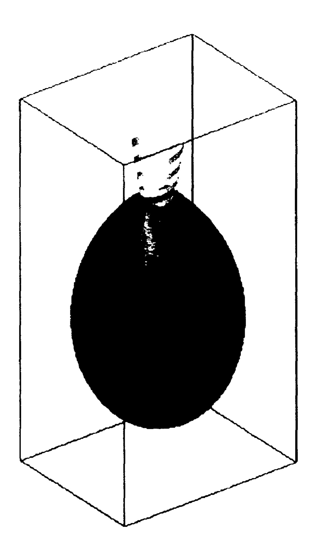
Fig 7. Polar plot of conical antenna at 500 Thz. Mathematically modeled by Dennis Prather at University of Delaware August 2004.
