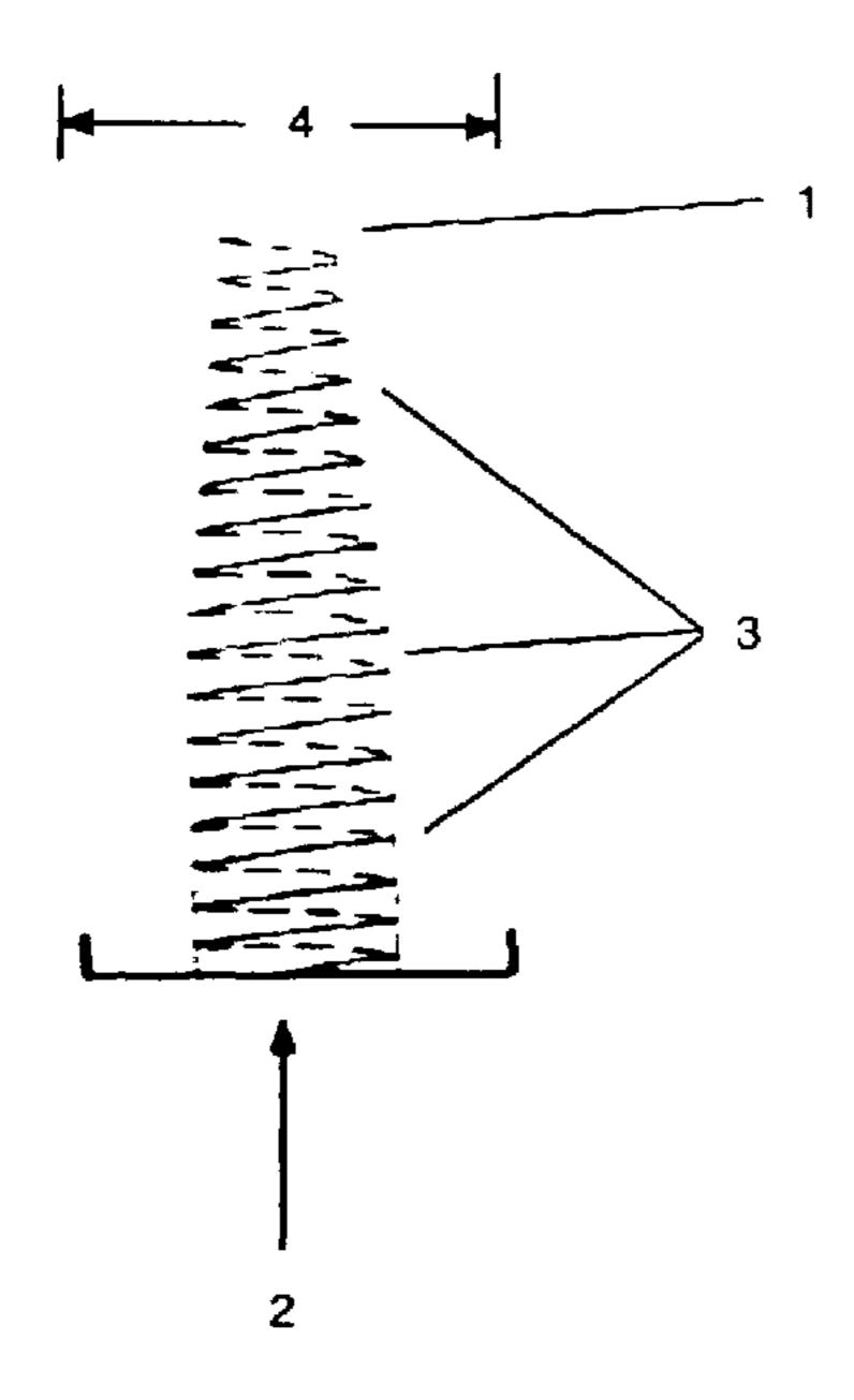
Fig 1: Color detecting pixel element in the form of a tapered conical antenna. Based on Johnson, Richard C., Antenna Engineering Handbook, 3<sup>rd</sup> edition, 1961. New York: McGraw-Hill. Page 13-13.
