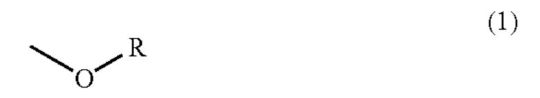
wherein R indicates an alkyl group having from 1 to 5 carbon atoms. The number of carbon atoms of the alkoxy group should be between 1 and 5 in order to obtain an EVOH resin having good melt extrusion stability, drawdown resistance, interlayer adhesion and gas-barrier properties. Preferably, the number of carbon atoms should be between 1 and 3, and is most preferably 1.
