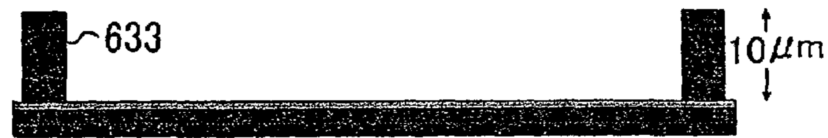
Fig. 16(b) Si DEPOSITION, ETCHING
