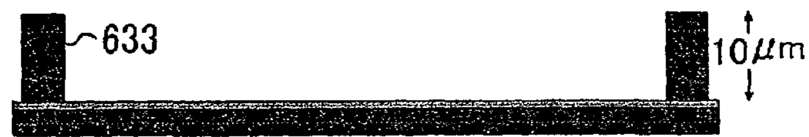
Fig. 16(b) Si DEPOSITION, ETCHING
