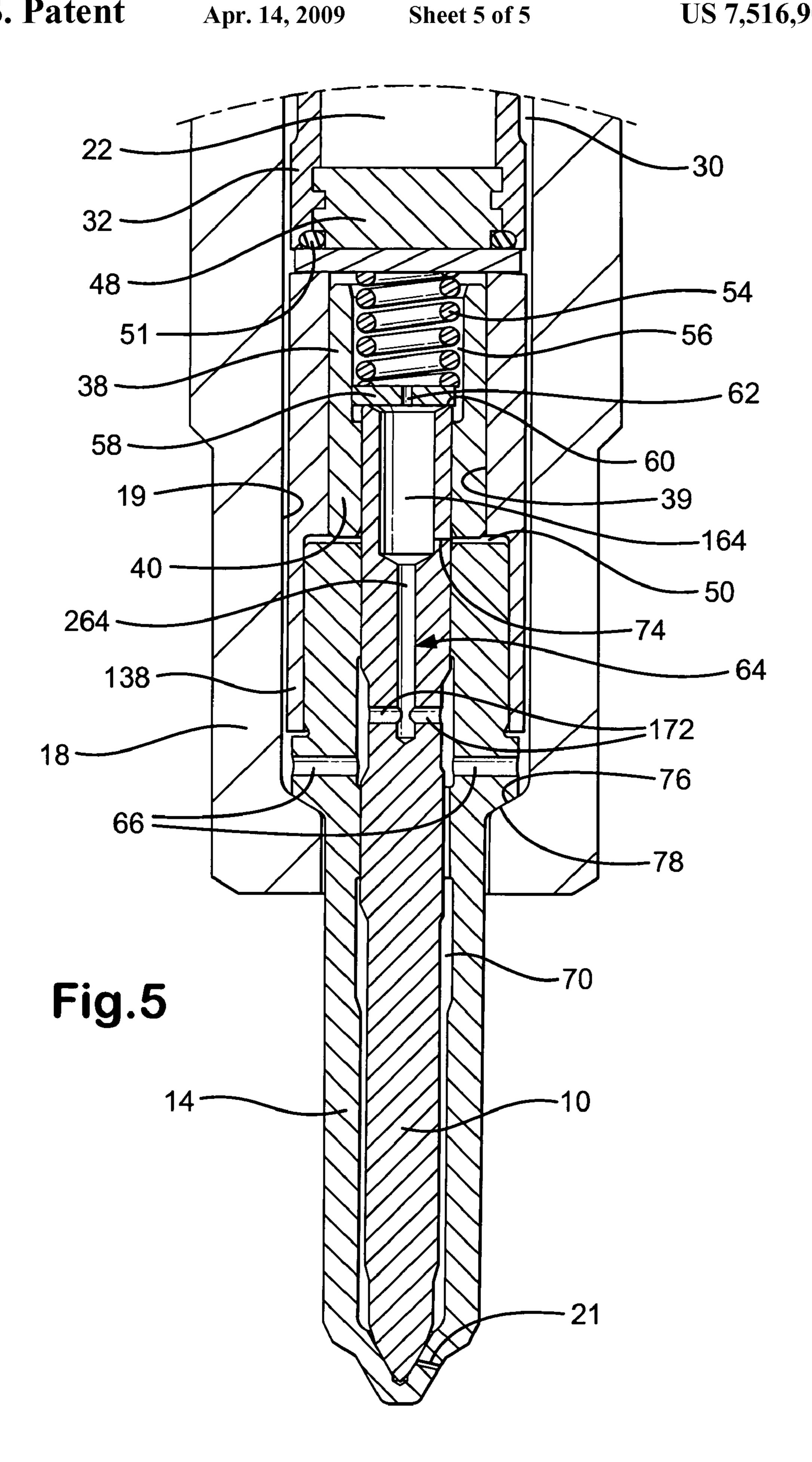
The present invention relates to a fuel injector for delivering fuel to a combustion space of a compression ignition internal combustion engine. In particular, but not exclusively, the invention relates to a fuel injector including a piezoelectric actuator for controlling movement of an injector valve needle.
