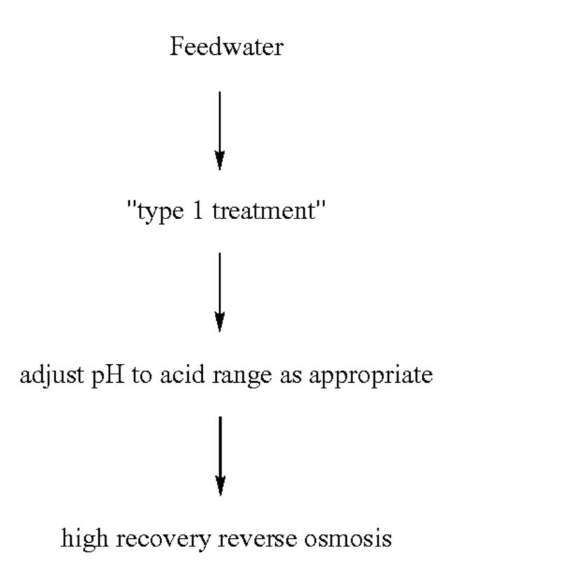
In the foregoing sequence, the term "type 1 treatment" is understood to encompass those standard RO pretreatments prior to conventional RO which would be deemed appropriate and necessary for the particular feedwater at hand by one skilled in the art. Such standard RO pretreatments are those
