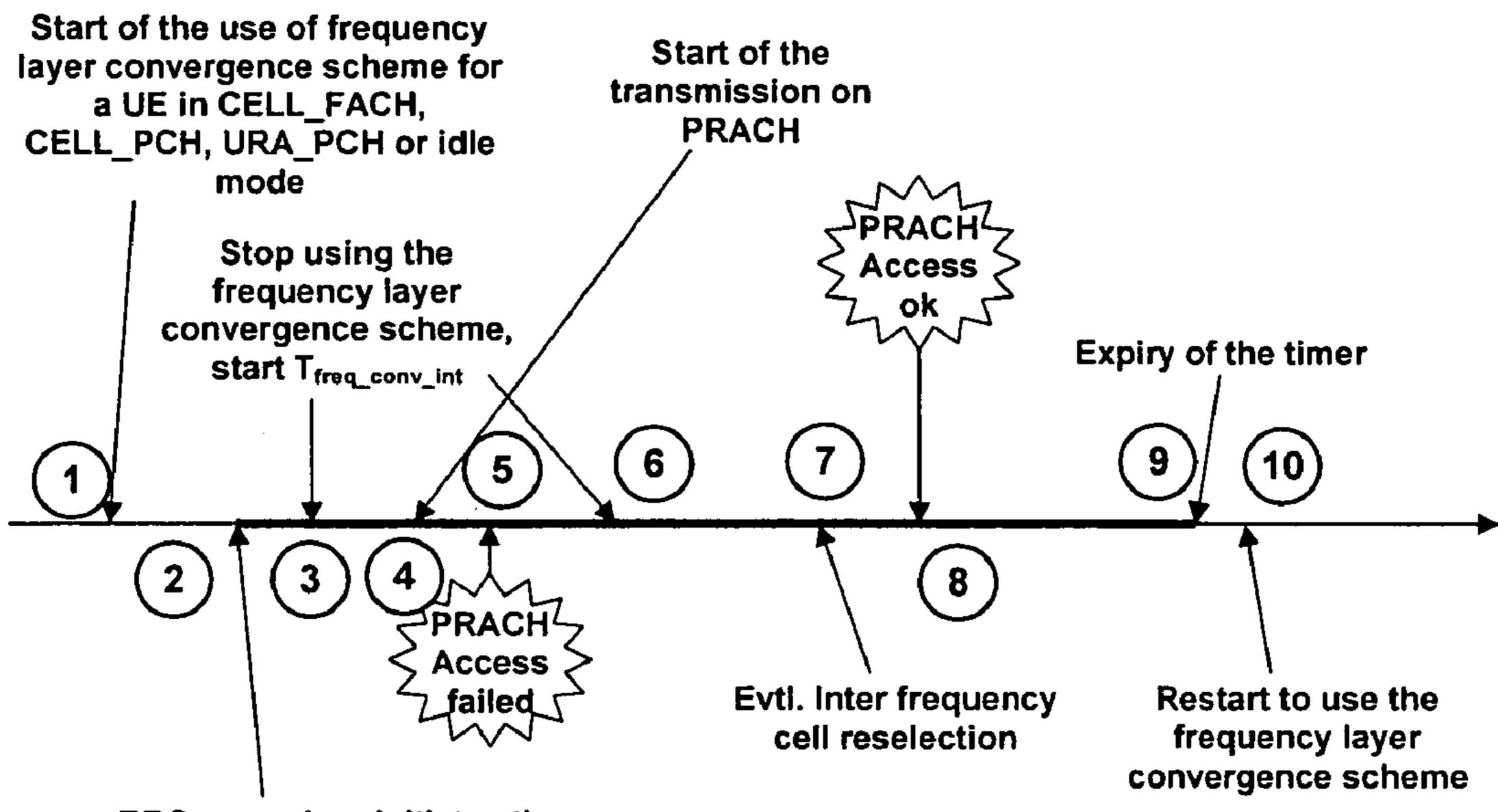
RRC procedure initiates the transmission of a message on the PRACH / start of data transmission / NAS initiates establishment of connection with CN domain with a given cause value / UE is ordered to select a cell ona given frequency.
