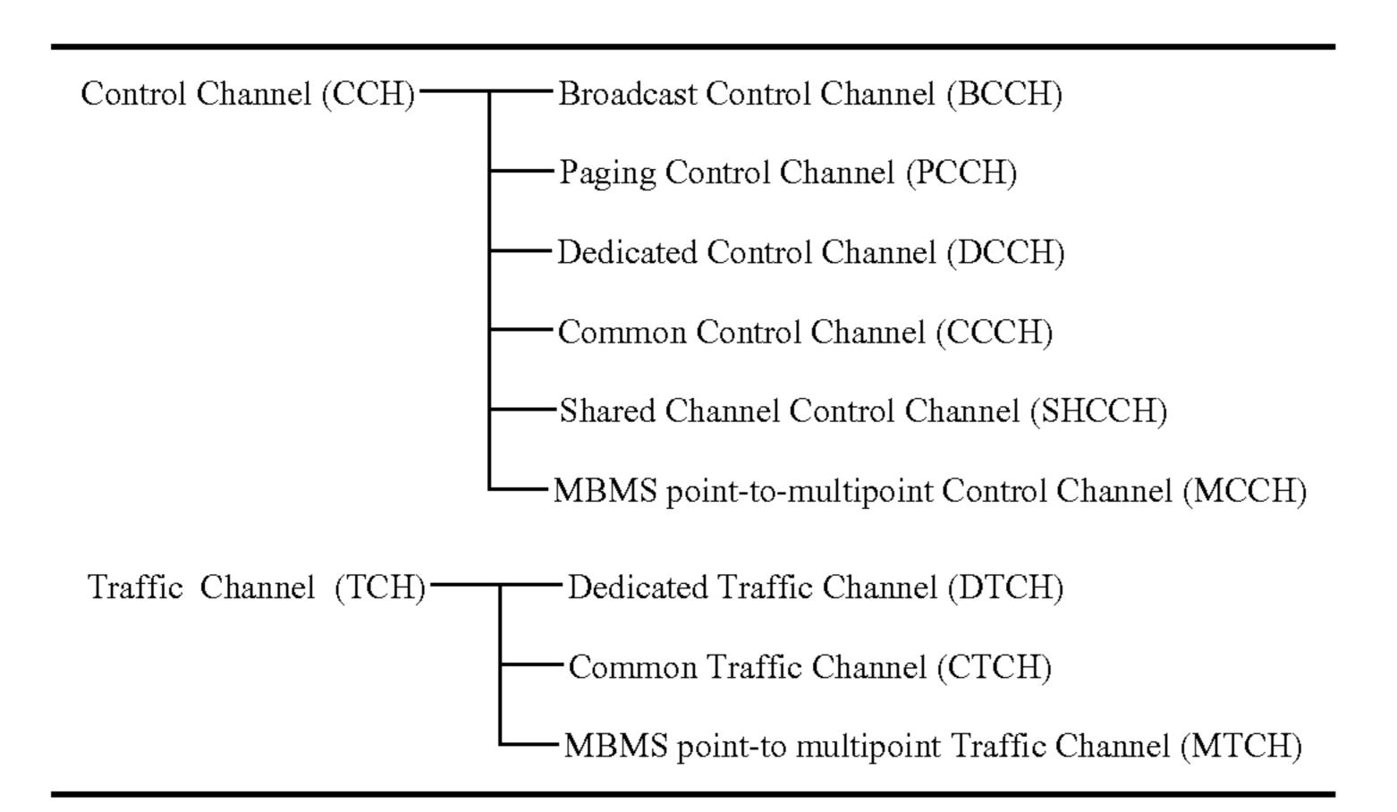
received from the upper layer, and transfers the BMC message to the RLC layer. The BMC messages are transferred from the RLC layer to the MAC layer through a logical channel, i.e., the CTCH (Common Traffic Channel). The CTCH is mapped to a transport channel, i.e., a FACH, which is mapped to a physical channel, i.e., a S-CCPCH (Secondary Common Control Physical Channel).
