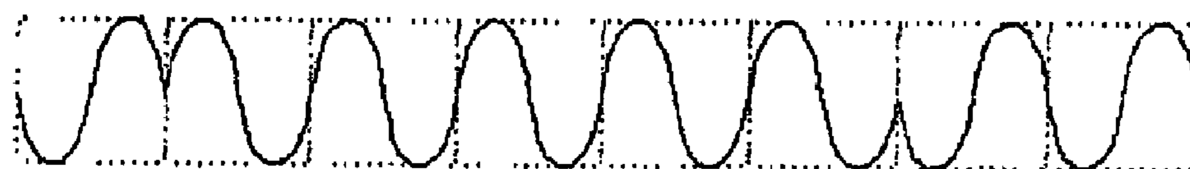
BPSK OR FSK PATTERN SIGNAL INDICATING BIT VALUE "1" OF ADDRESS DATA
