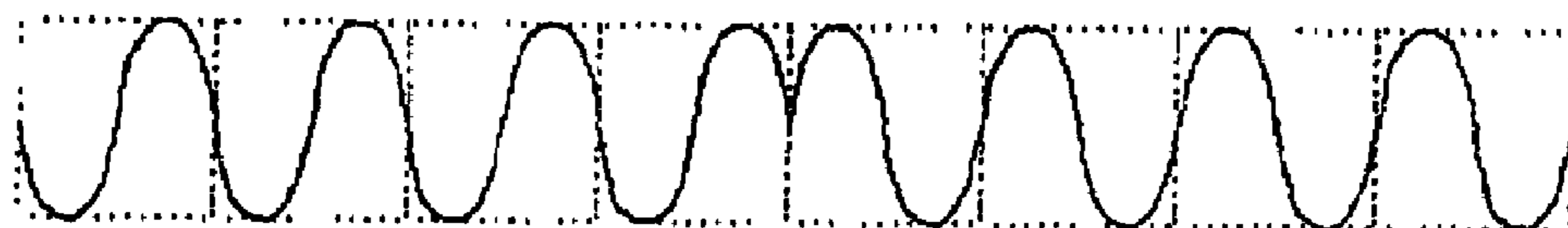
BPSK PATTERN SIGNAL INDICATING START OF ADDRESS DATA
