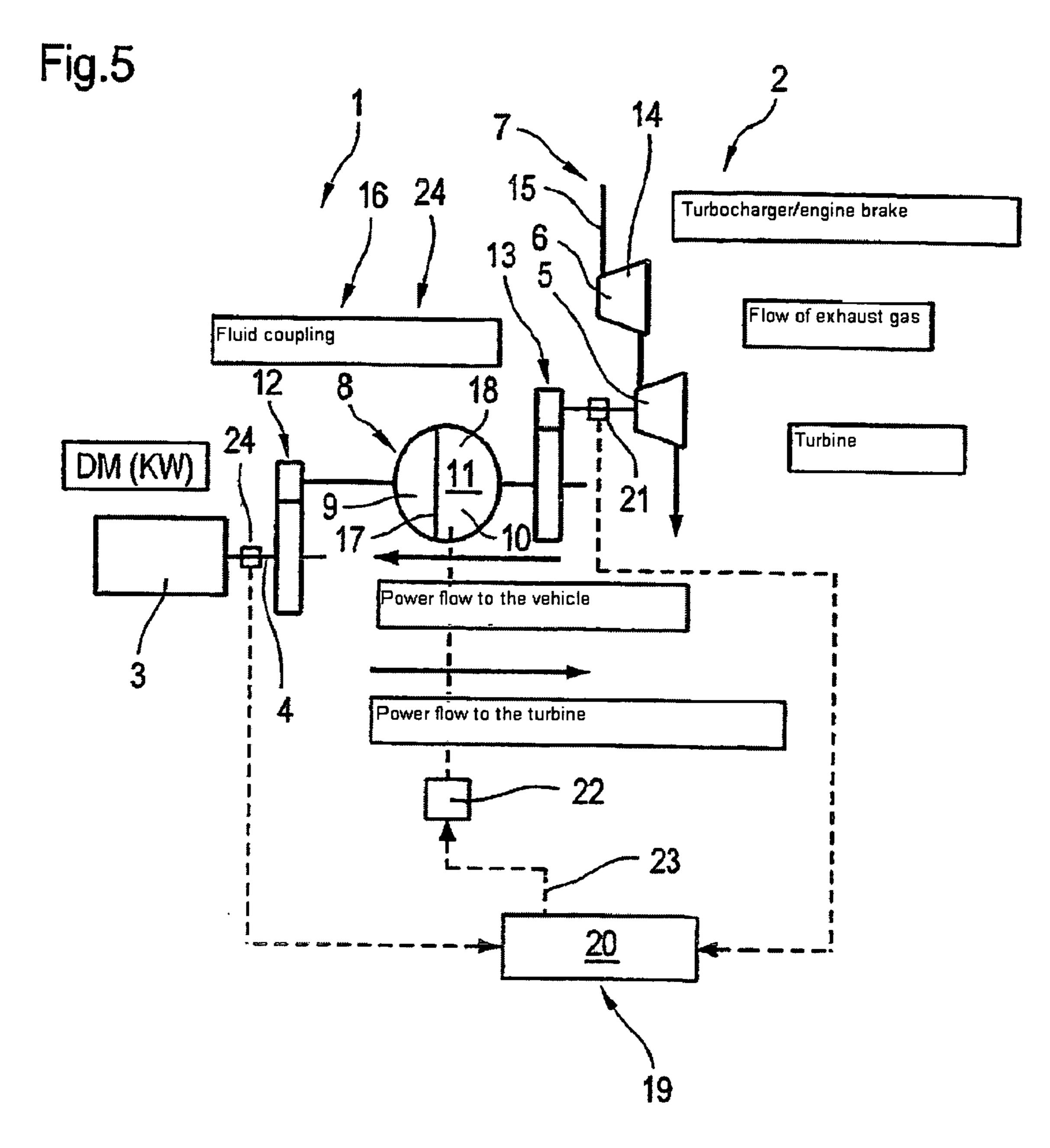
DM (KW) = Driving machine (crankshaft)
