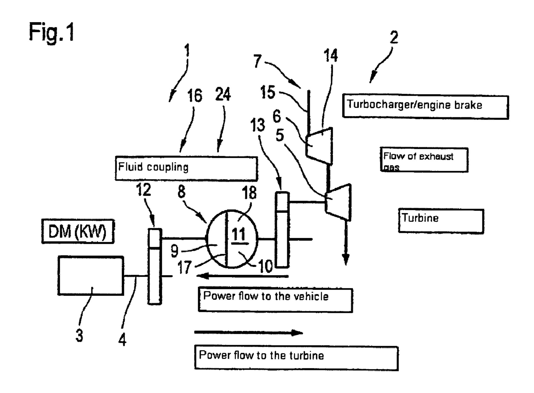
DM (KW) = Driving machine (crankshaft)
