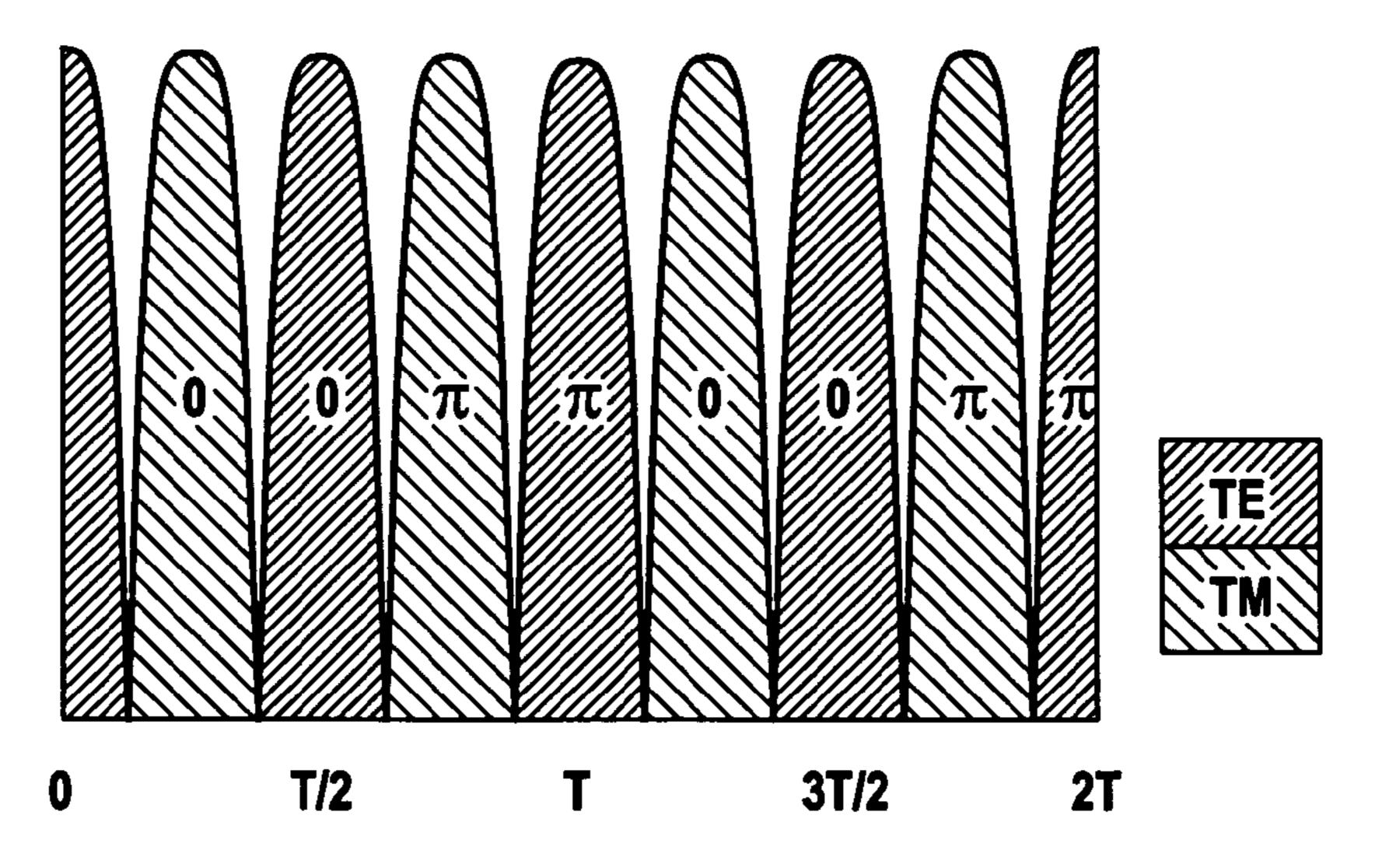
Pulses stream at  $4F_{clock}$  after OTDM (Coding section omitted for demonstration)
