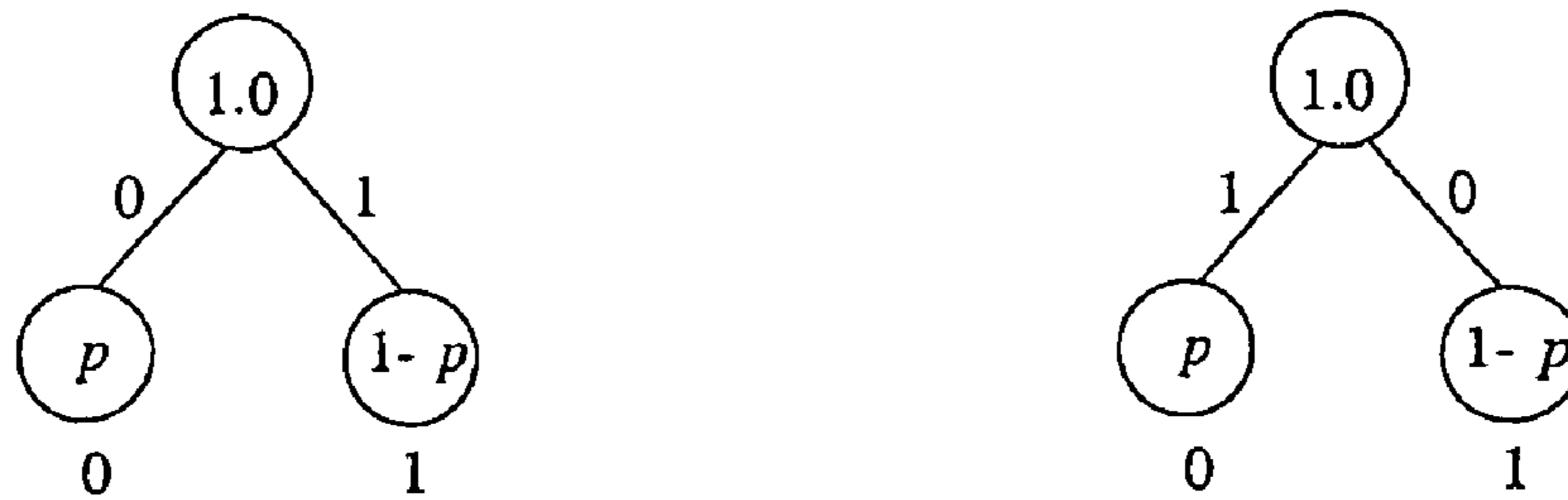
(a) Huffman tree labelled using the assignment 0 to the left and 1 to the right.
