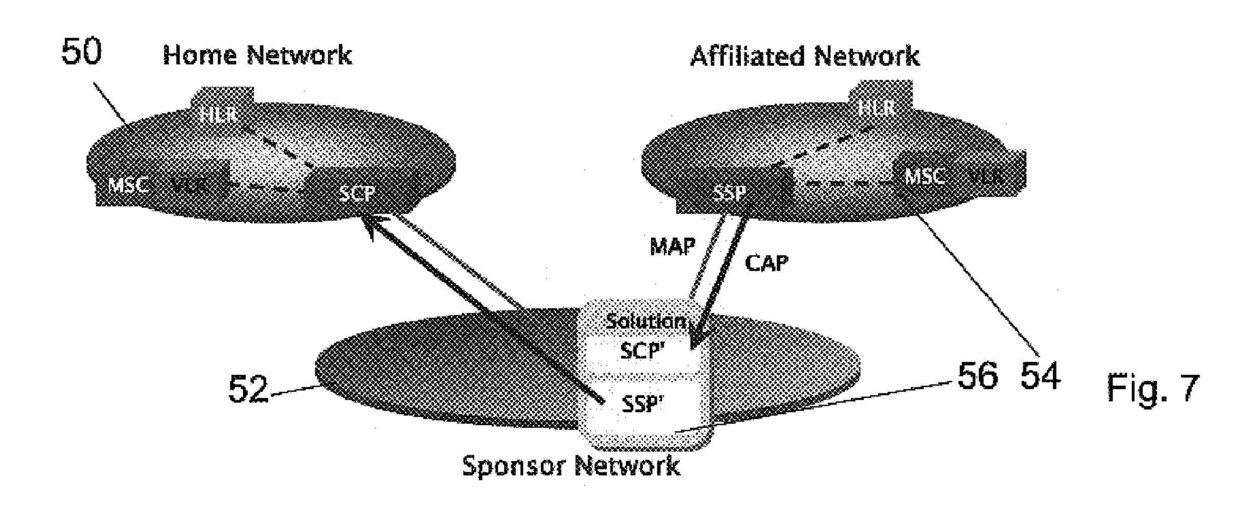
The CAMEL triggers will be delivered to the solution platform, located at the sponsored network, then delivered to the home network. The green line stands for the MAP signaling, which is routed via the sponsored network too.
