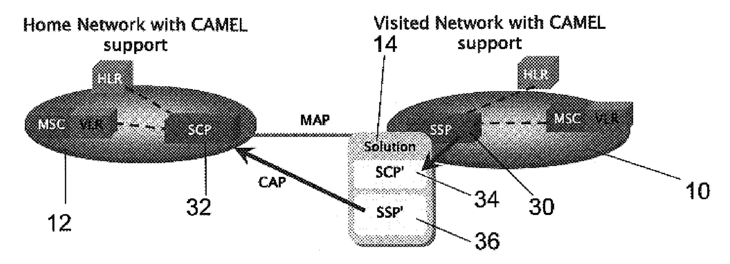
The CAMEL triggers will be delivered first to the SCP', being a part of the solution, then delivered to the home network by SSP', also part of the solution. (CAP: CAMEL Application Protocol)
