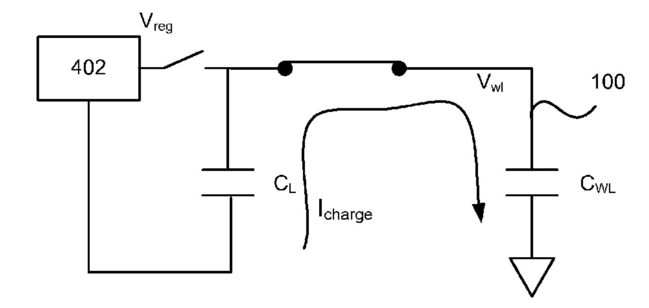
$$\Delta V_{wl} = \frac{C_1}{C_1 + C_2} V_{supply}; \text{ if } C_1 = C_2, \text{ then } V_{wl} = .5 V_{supply}$$
