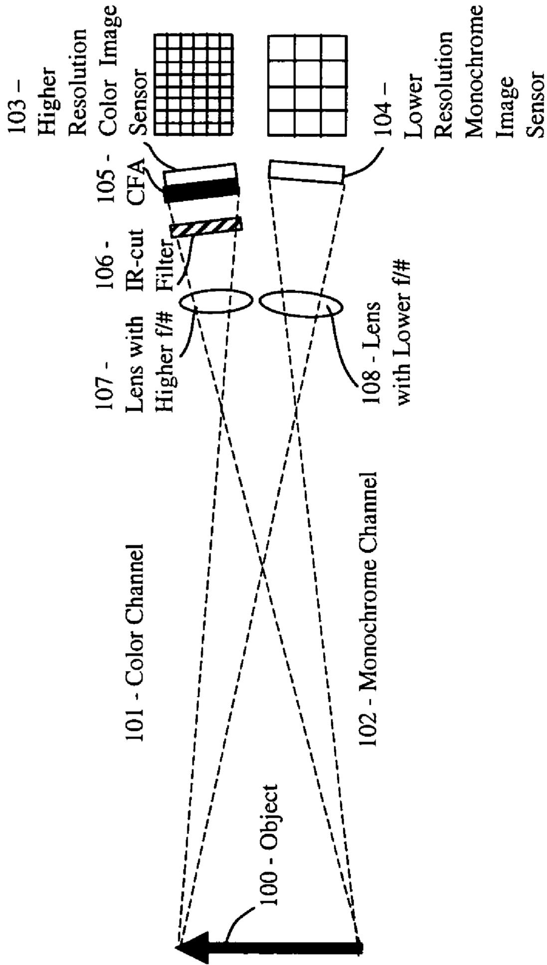
Figure 1. Dual spectral band network camera head
