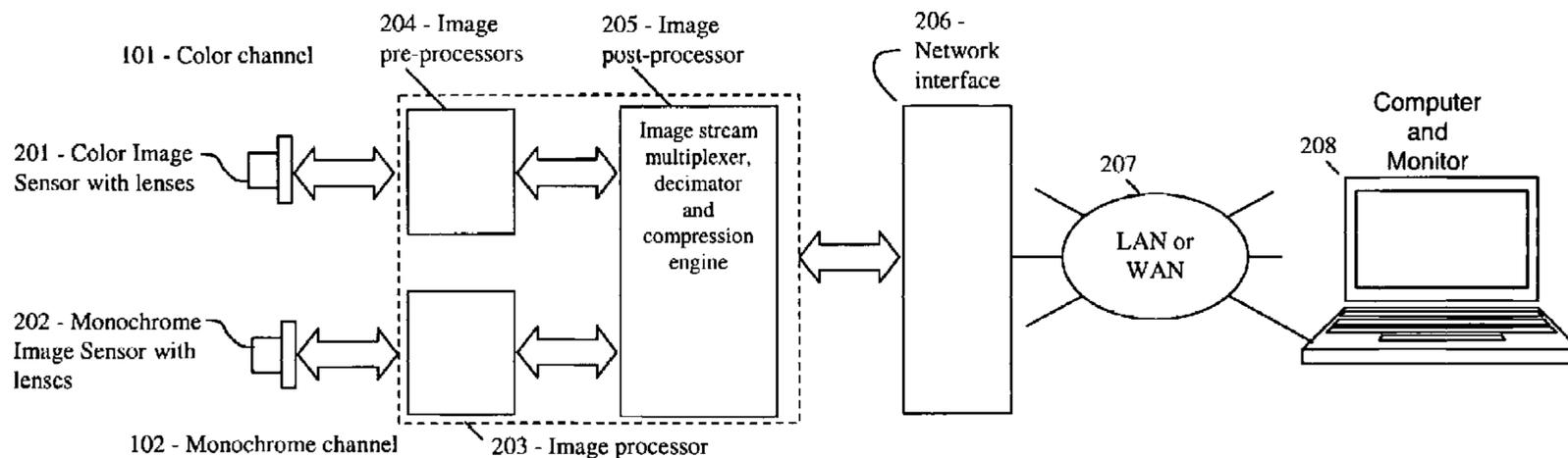
Block diagram of Dual Spectral Band Network Camera
