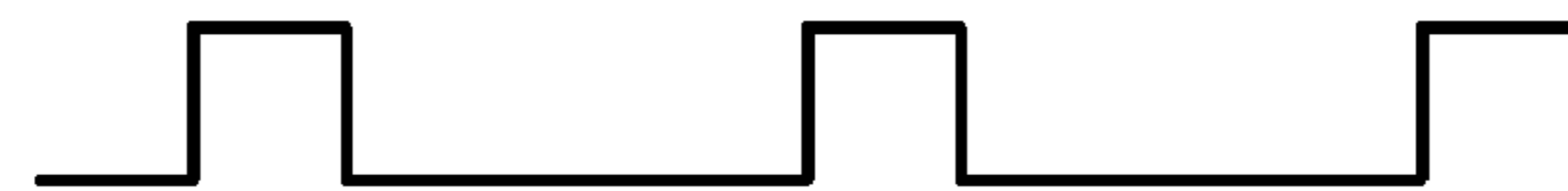
PFM, pulse frequency modulation (aka pulse skipping)
