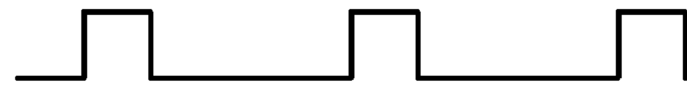
PFM, pulse frequency modulation (aka pulse skipping)
