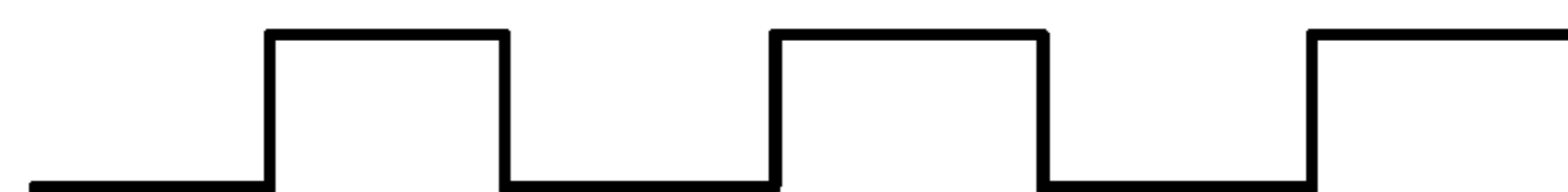
PWM, pulse width modulation
