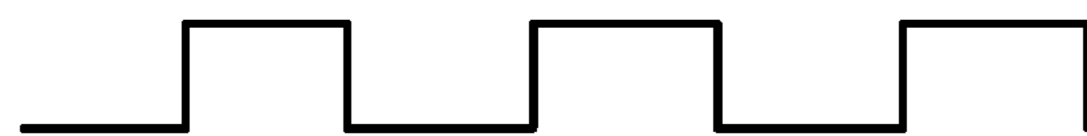
PWM, pulse width modulation
