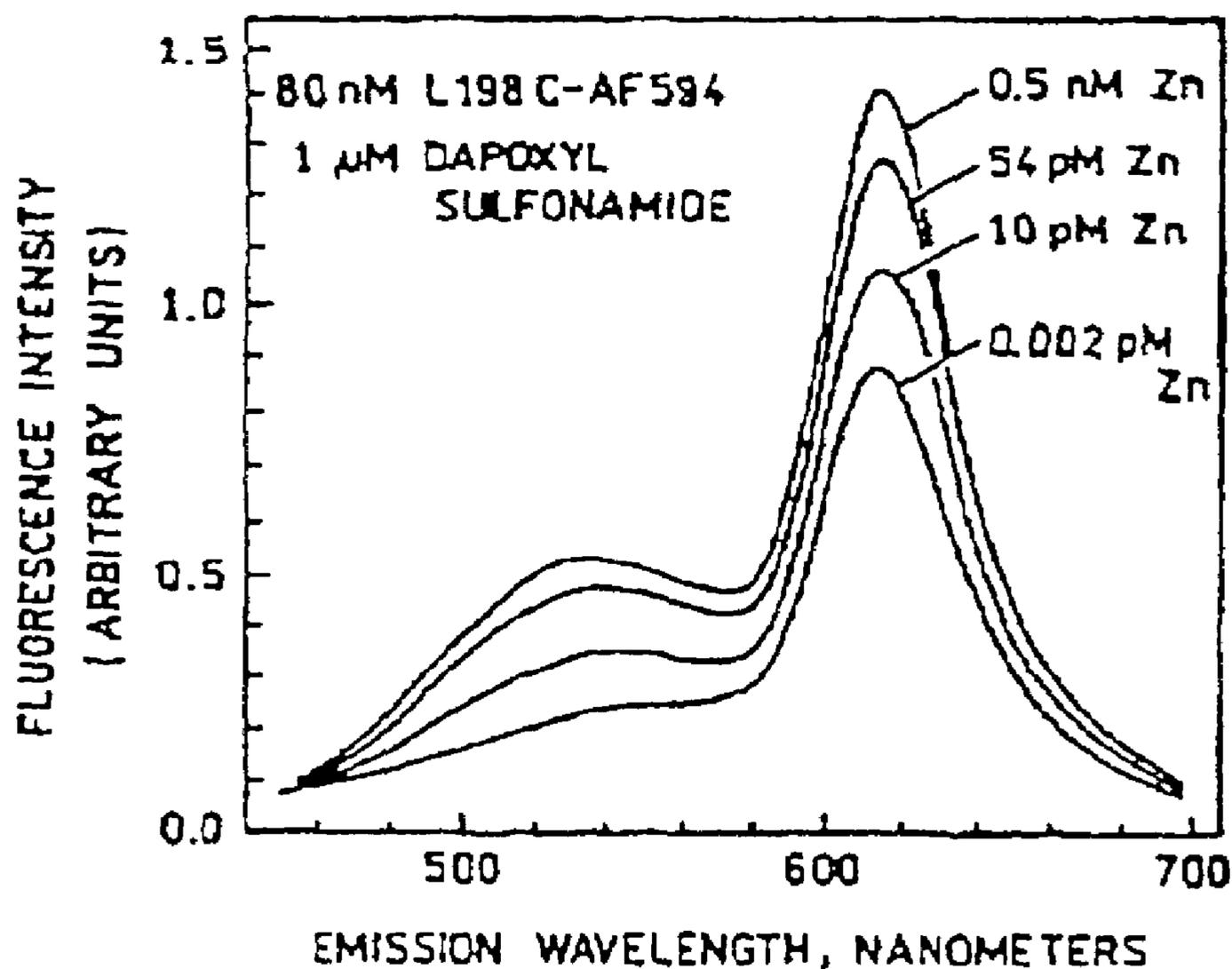
Fig. 4 Emission spectra of 80 nM apoL198C-Alexa Fluor 594 and 1  $\mu$ M Dapoxyl sulfonamide in the presence of solutions buffered at (in ascending order at 610 nm) 0.002, 10, 54, and 0.5 nM free Zn(II); excitation at 365 nm.
