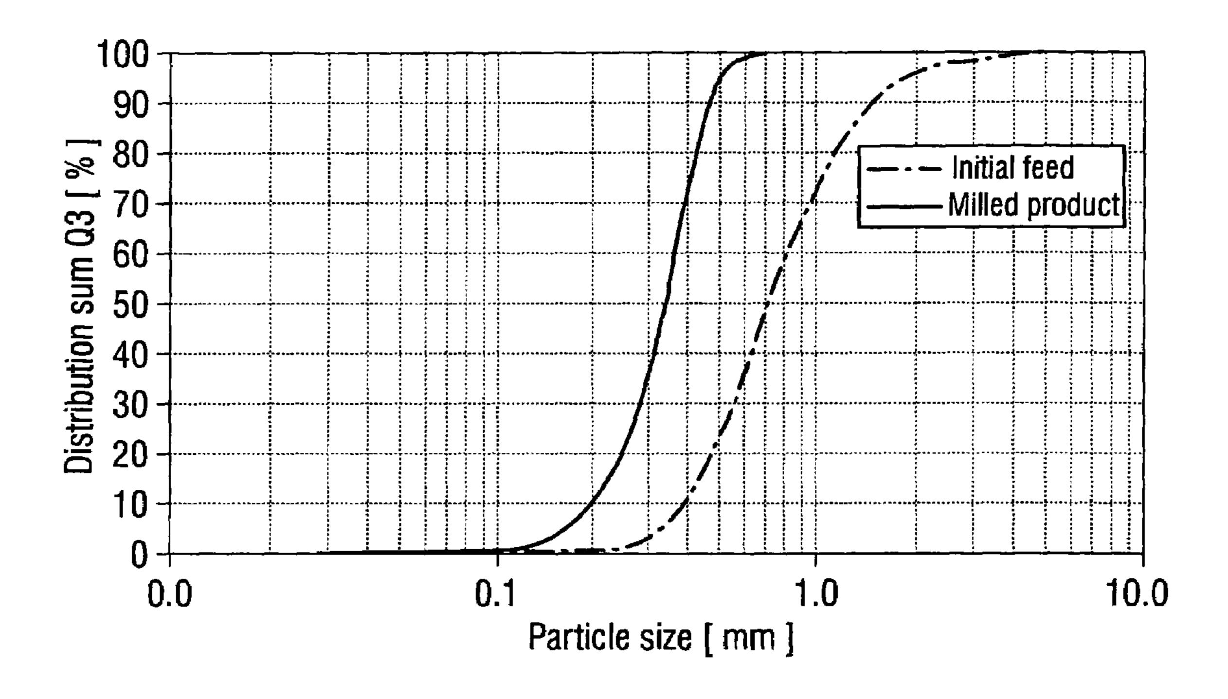
Mass - referenced distribution densities of feed material (silicon granules) and milled product (silicon seed particles)
