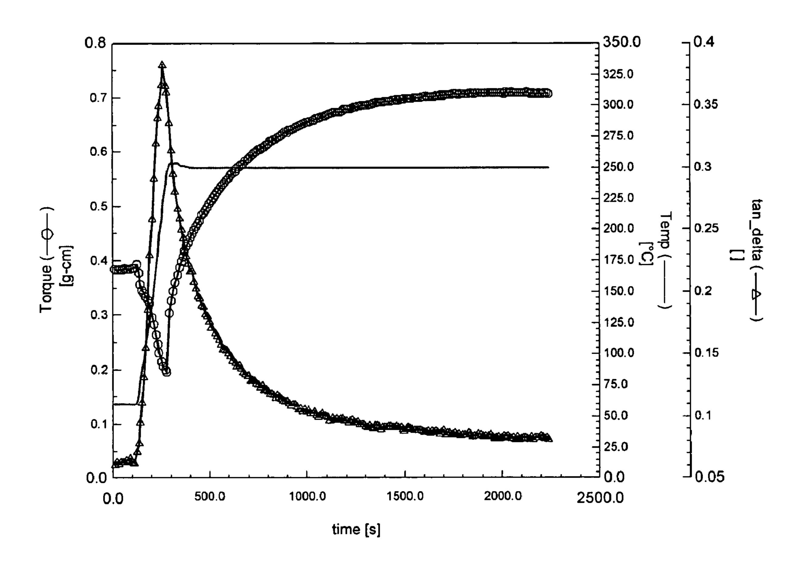
Figure 2. Curing kinetics obtained at 250°C (Example 4)
