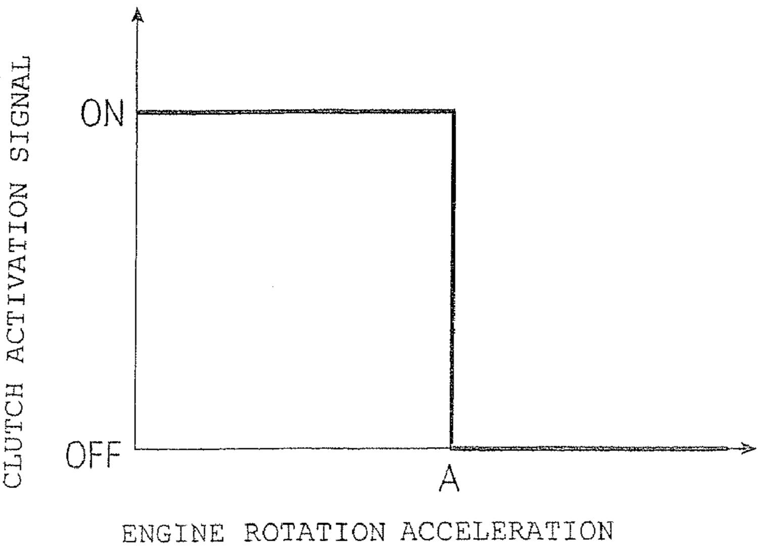
ENGINE ROTATION ACCELERATION (ACCELERATION OPENING ACCELERATION)
