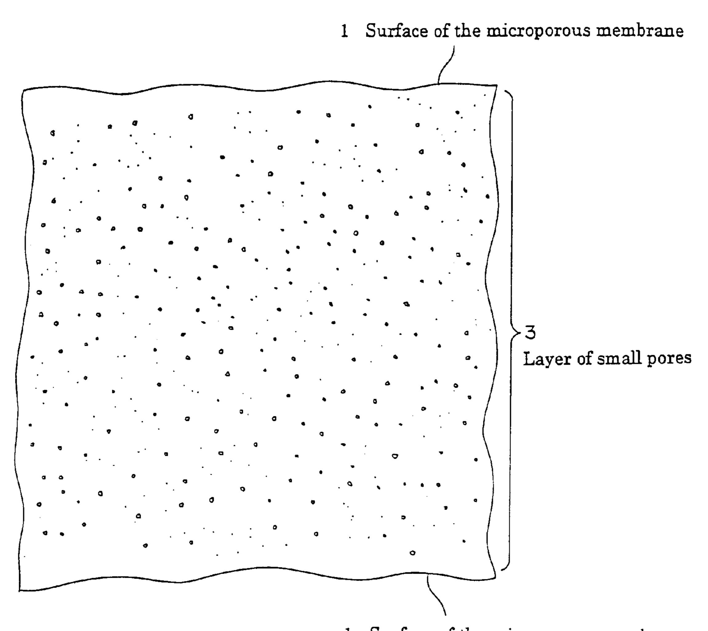
1 Surface of the microporous membrane
