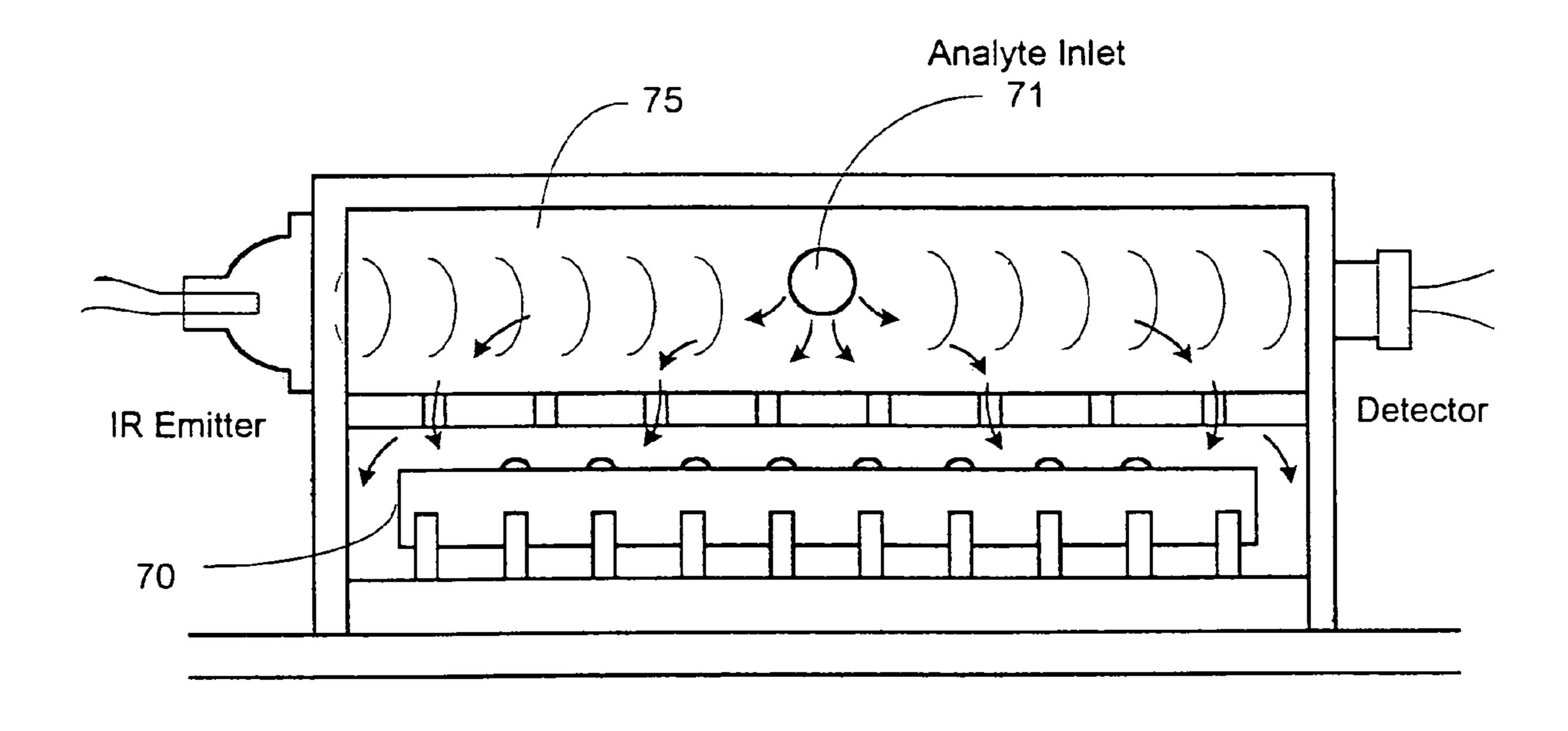
Section View: Sensor Chamber
