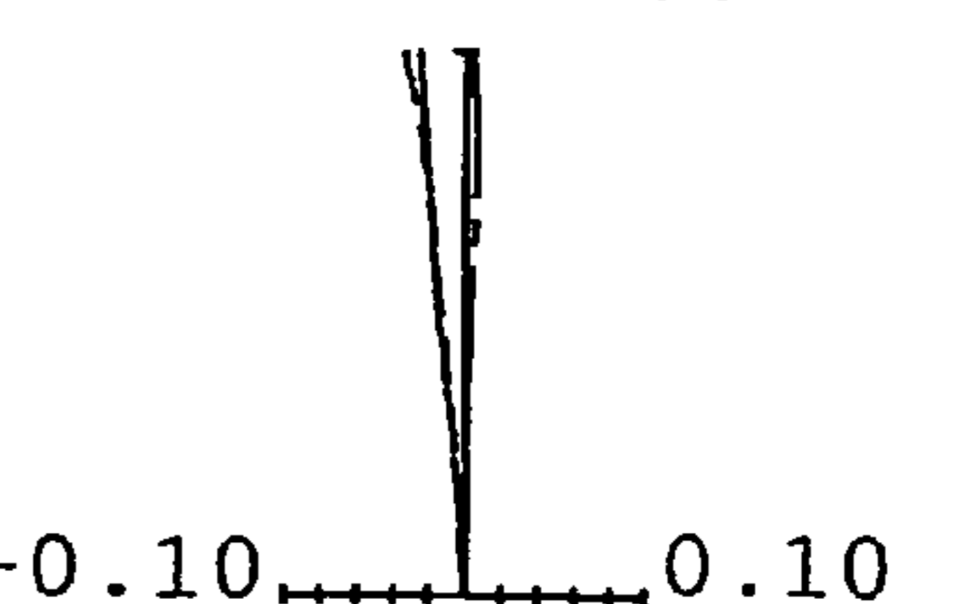
FIG. 9L CHROMATIC ABERRATION OF MAGNIFICATION FL=560 FIY 11.00
