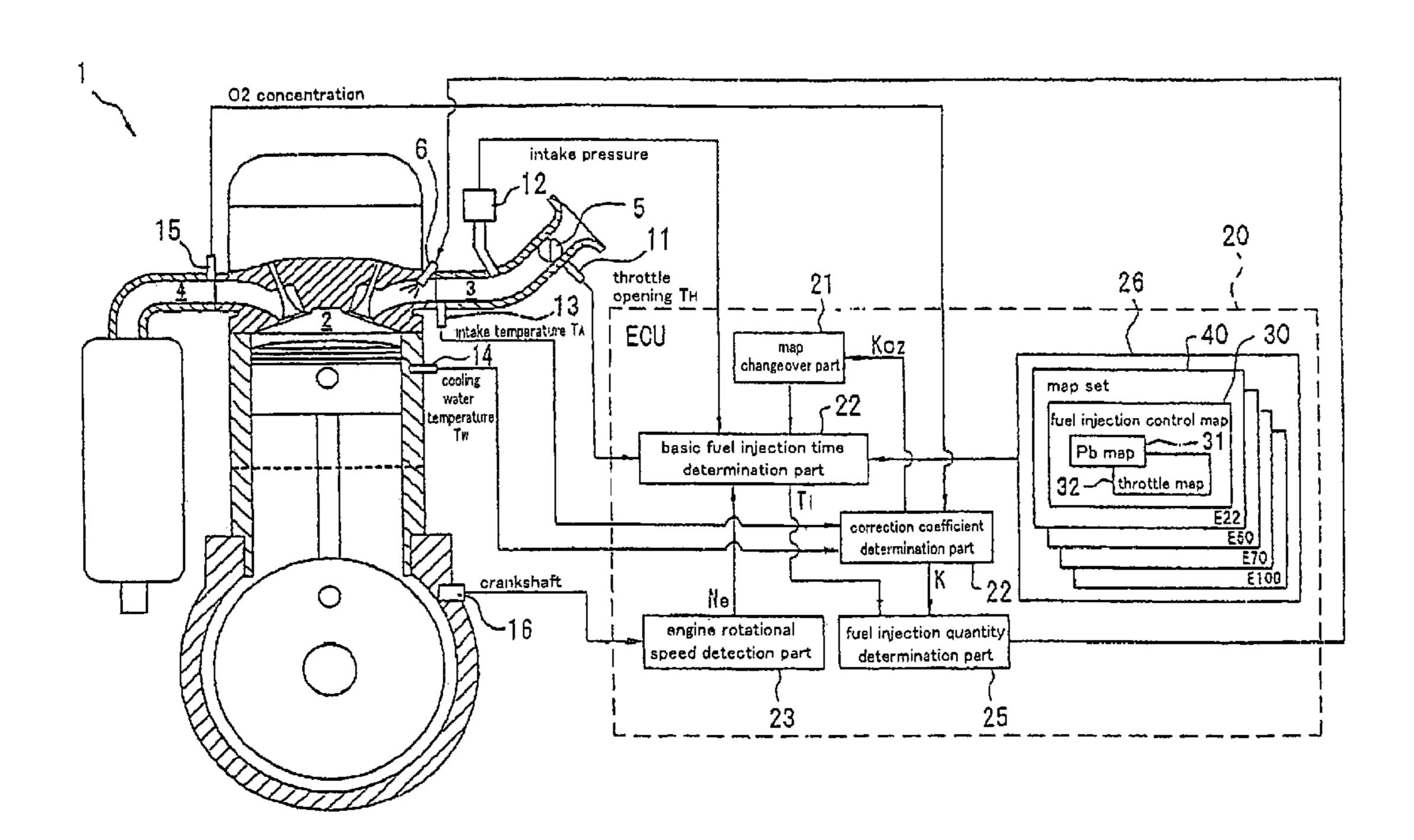
fuel injection control map 25 fuel injection quantity correction coefficient map changeover part fuel injection time part angine rotational speed detection part determination pressure
