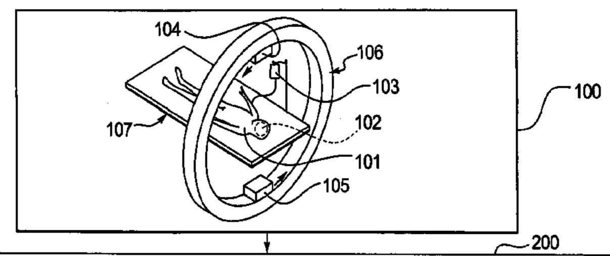
AT FIRST ROTATIONAL POSITION OF RAY SOURCE FOR A FIRST ROTATION AT A FIRST TIME POINT A FIRST IMAGE IS OBTAINED, AND AT THE FIRST ROTATIONAL POSITION FOR ANOTHER ROTATION AT A SECOND TIME POINT A SECOND IMAGE IS OBTAINED, THE FIRST AND SECOND IMAGES BEING DIFFERENT FROM ONE ANOTHER IN VIEW OF FLOWING CONTRAST AGENT
