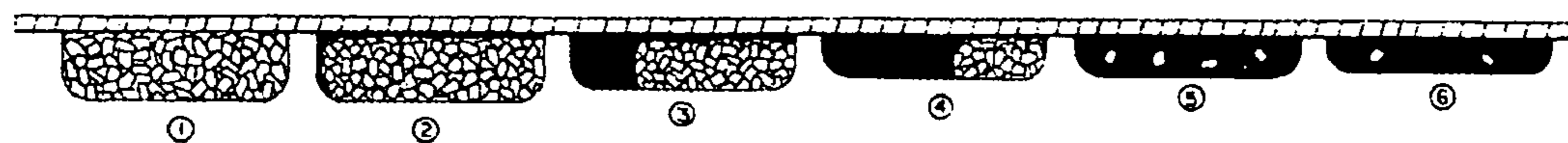
Fig. 3: Melting In Screw Channel
