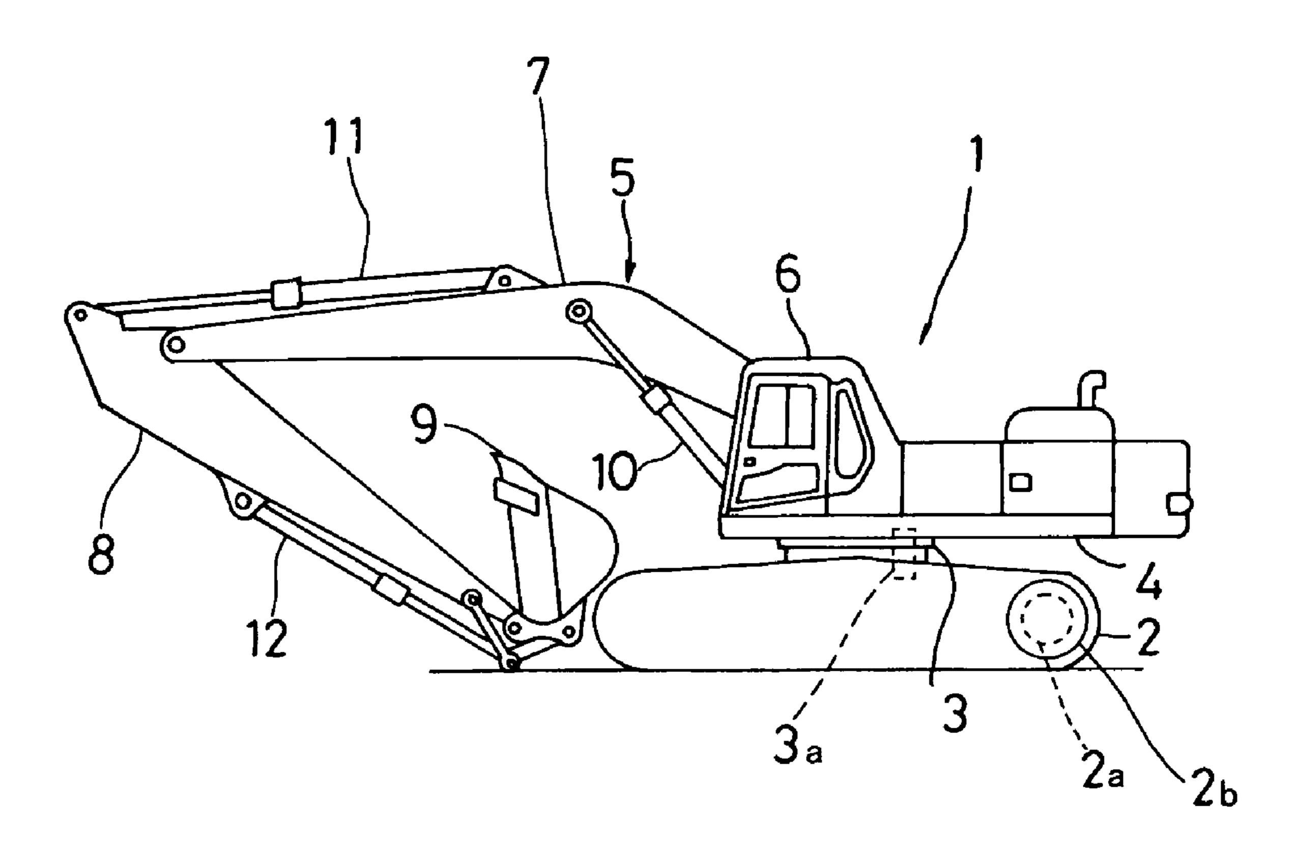
FIG. 2 boom cylinder 10 \ arm cylinder 11 bucket cylinder 12 hydraulic actuator hydraulic motor for rotation 3a hydraulic motor for traveling 2a 18 control valve self pressure reducing valve 16 34~ 35. servo valve 22~ 28~ LS valve 29/ PC valve 30 ~ 21a-LS-EPC PC-EPC valve valve 32memory unit controller
