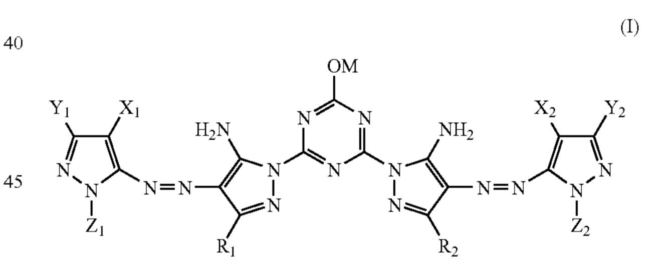
where  $X_1$ ,  $X_2$ ,  $Y_1$ , and  $Y_2$  are each a hydrogen atom or a cyano group,  $Z_1$  and  $Z_2$  are each a substituent having an aromatic ring,  $R_1$  and  $R_2$  are each an alkyl group, and M is a metal atom;
