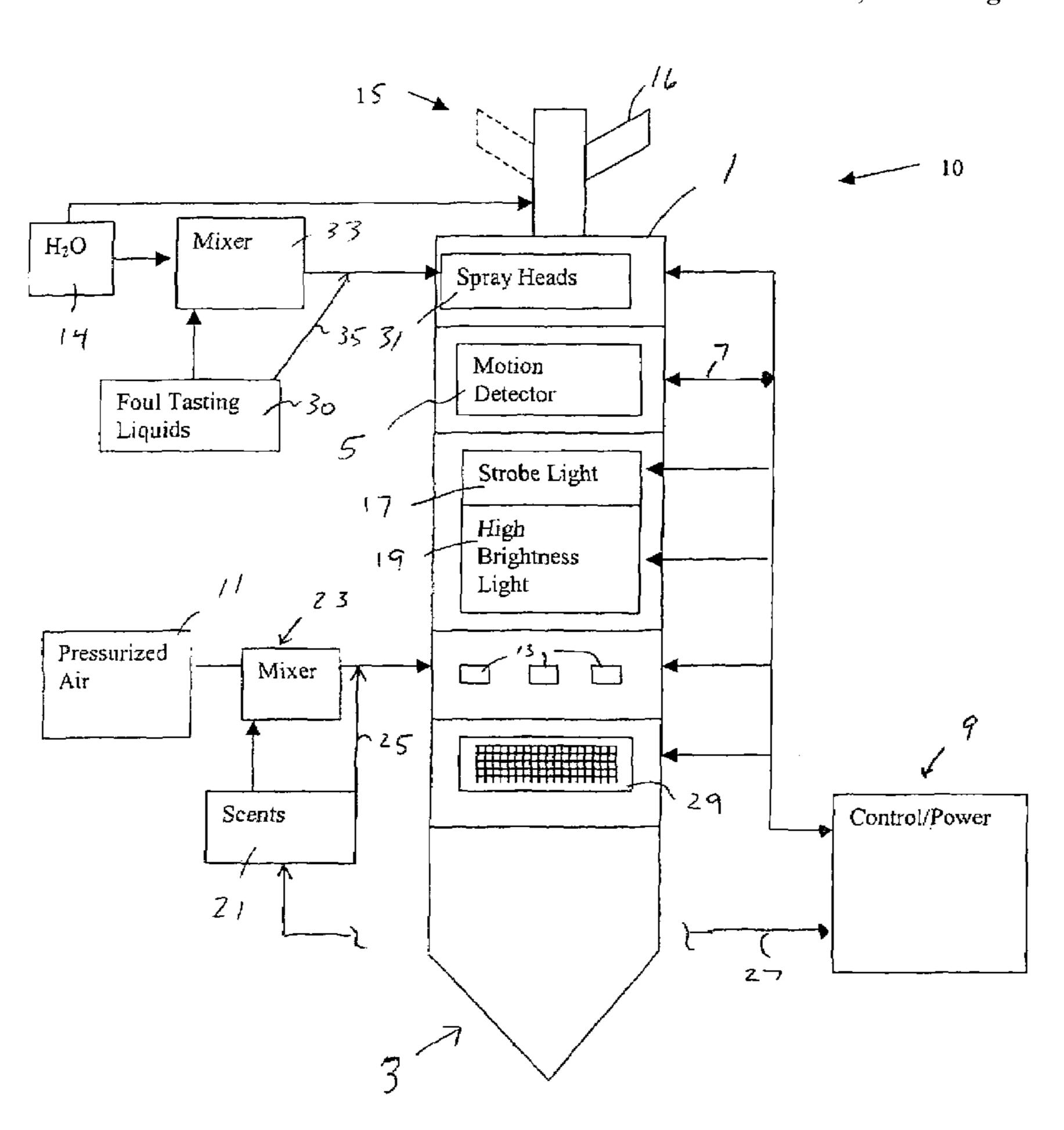
F19. 1 10 33 Mixer  $H_2O$ Spray Heads 35 31 14 Motion Detector Foul Tasting 1~30 Liquids 5 Strobe Light High Brightness 19 Light Pressurized Mixer Air 29 Scents Control/Power 2つ
