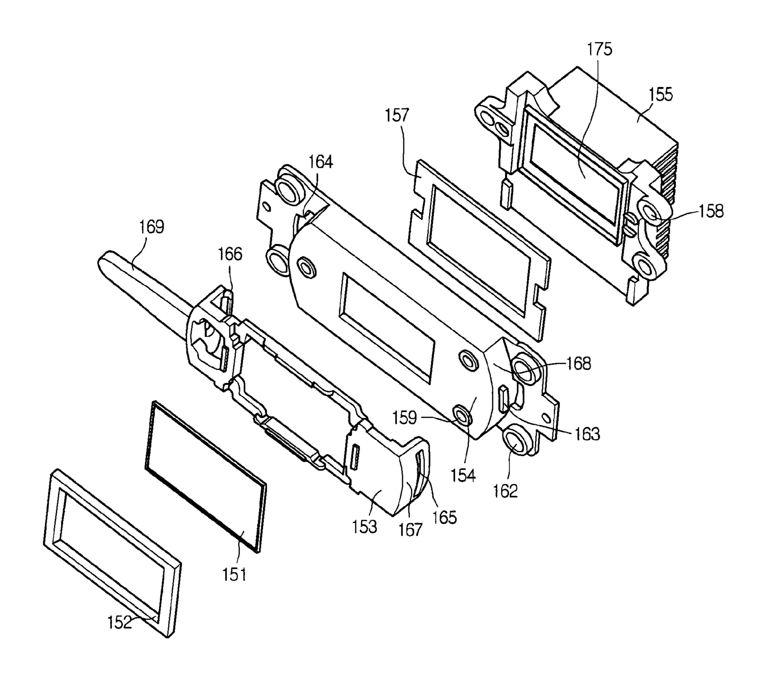
LCOS PANEL ASSEMBLY OF PROJECTION SYSTEM AND IMAGE MATCHING METHOD HAVING QUARTER WAVE PLATE HOLDER ROTATABLY SUPPORTED ABOUT PANEL SUPPORT BY RESPECTIVELY SLOTS AND PROTRUSIONS
